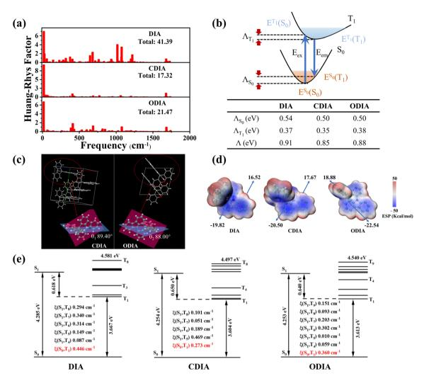
Fig. 3 (a) The Huang–Rhys factors *versus* frequencies of DIA, CDIA, and ODIA. (b) Theoretical estimation of the total reorganization energies (Δ). (c) The molecular geometries of CDIA and ODIA single crystals. (d) Calculated ESP distribution of DIA, CDIA, and ODIA. (e) Calculated energy diagram and spin–orbit coupling (SOC) matrix elements (ξ).
