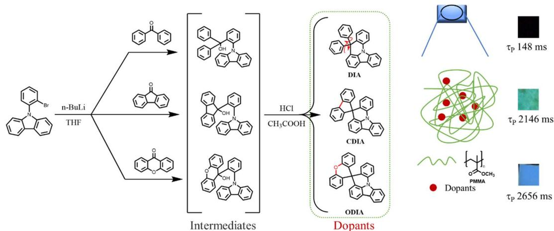
Fig. 1 Chemical strategies to prepare polymer-based RTP materials.
