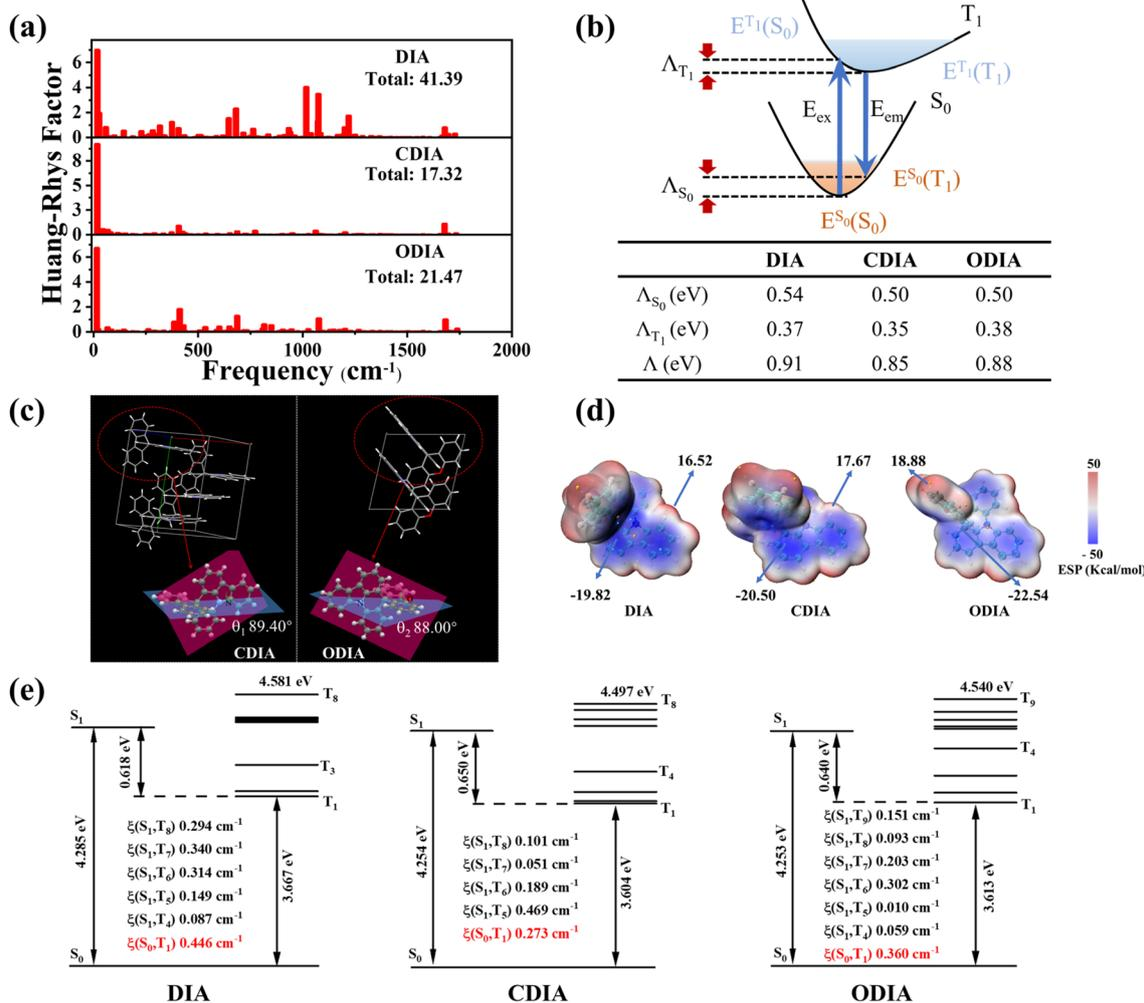
Fig. 3 (a) The Huang–Rhys factors versus frequencies of DIA, CDIA, and ODIA. (b) Theoretical estimation of the total reorganization energies ( $\Lambda$ ). (c) The molecular geometries of CDIA and ODIA single crystals. (d) Calculated ESP distribution of DIA, CDIA, and ODIA. (e) Calculated energy diagram and spin–orbit coupling (SOC) matrix elements ( $\xi$ ).
