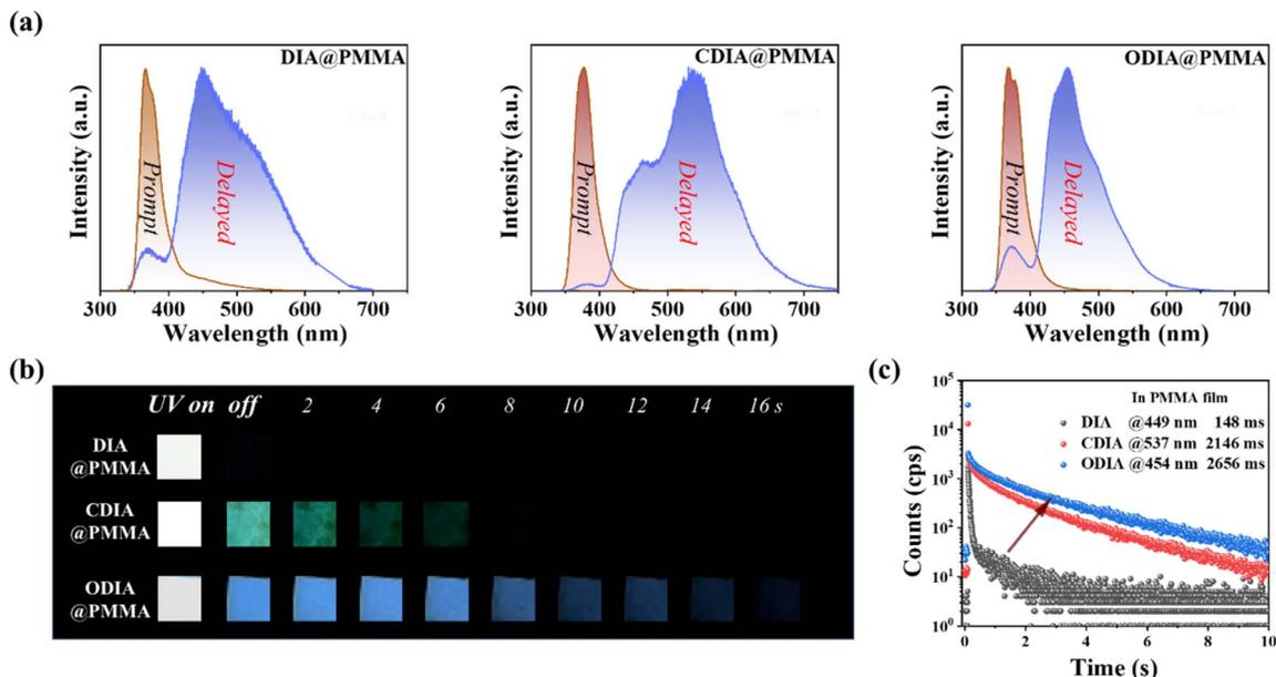
Fig. 2 (a) The prompt and delayed PL spectra of DIA@PMMA, CDIA@PMMA, and ODIA@PMMA under 280 nm light excitation. Due to the overlap between the 365 nm excitation peak and the fluorescence peak, the test was conducted using 320 nm excitation. (b) Room temperature PL photographs of DIA, CDIA, and ODIA in PMMA after removing 365 nm UV light ( $3 \text{ mW cm}^{-2}$ ). (c) The time-resolved RTP decay curves and fitted long-component RTP lifetimes under 365 nm light excitation.
