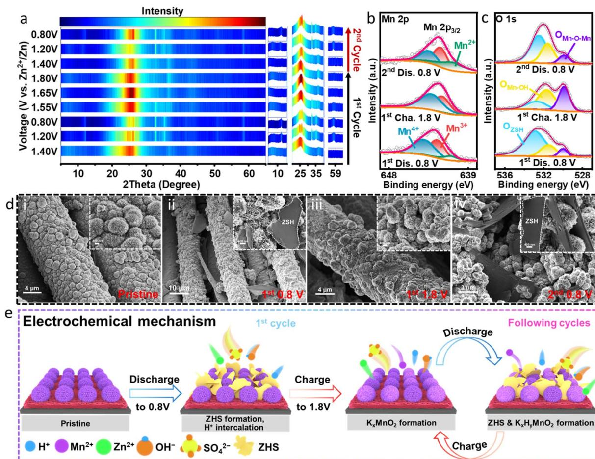
Fig. 5 (a) *Ex situ* XRD patterns of the MNSMO@CC electrode collected at specific voltage states. *Ex situ* XPS of (b) Mn 2p and (c) O 1s, and (d) *ex situ* SEM of the MNSMO@CC electrode in different voltage states. (e) Schematic diagram of the aqueous Zn/MNSMO@CC battery storage mechanism.
