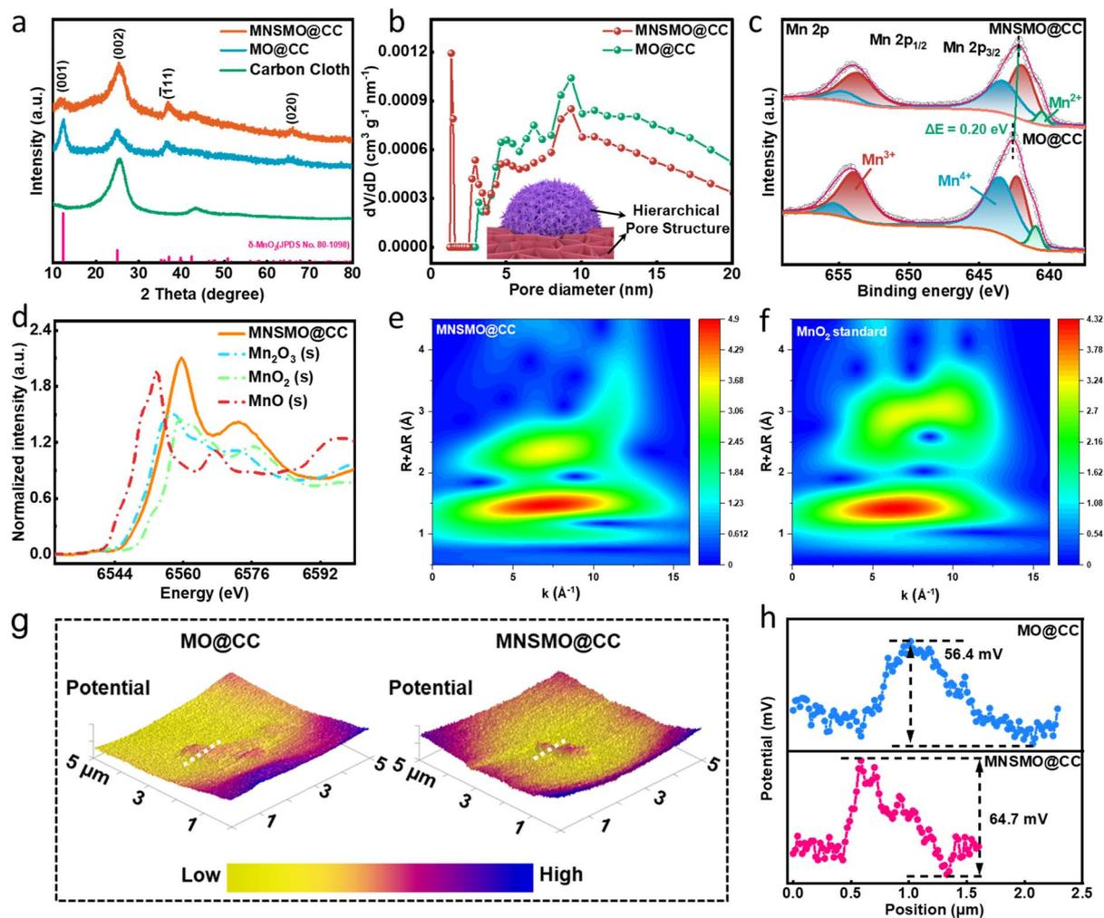
Fig. 2 (a) XRD pattern, (b) corresponding pore size distribution, and (c) high-resolution XPS spectra of Mn 2p of MNSMO@CC and MO@CC. (d) XANES spectra of MNSMO@CC and three standard oxides ( $\text{MnO}$ ,  $\text{Mn}_2\text{O}_3$ , and  $\text{MnO}_2$ ). (e and f) EXAFS wavelet transformation contour plots of MNSMO@CC and standard  $\text{MnO}_2$ . (g) 3D CPD contour projects and (h) the corresponding line-scan CPD distribution curves of MNSMO@CC and MO@CC.
