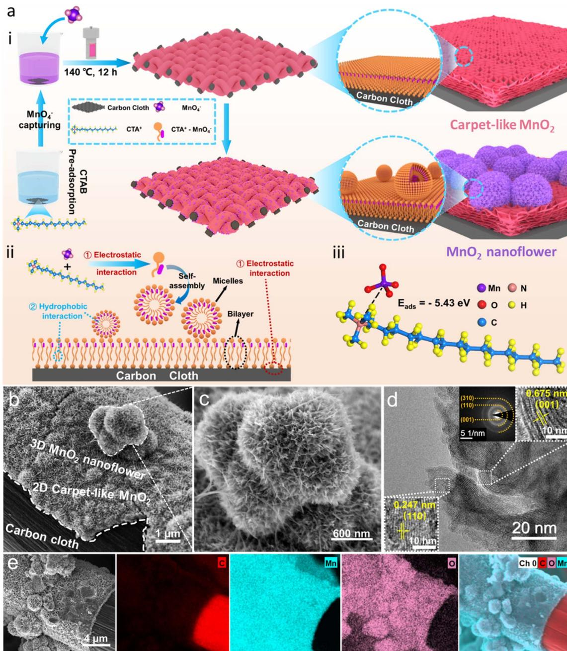
Fig. 1 (a) (i) The synthesis of MNSMO@CC, (ii) the molecular mechanism during the reaction, (iii) the adsorption energy of the  $\text{CTA}^+-\text{MnO}_4^-$  molecule. (b and c) SEM images of MNSMO@CC. (d) TEM image and SAED pattern of MNSMO@CC. (e) EDS mapping images of MNSMO@CC.
