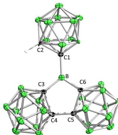
Fig. 2 Single crystal structure of complex **1** in the solid state. The hydrogen atoms were omitted for clarity. Thermal ellipsoids are drawn at the 50% probability level. Selected bond lengths [Å] and angles [°]: B–C1 1.558(2), B–C3 1.5966(16), B–C6 1.5966(16), C3–C4 1.6554(16), C4–C5 1.537(2), C5–C6 1.6554(16), C1–B–C3 124.55(7), C1–B–C6 124.55(7), C3–B–C6 110.74(14).
