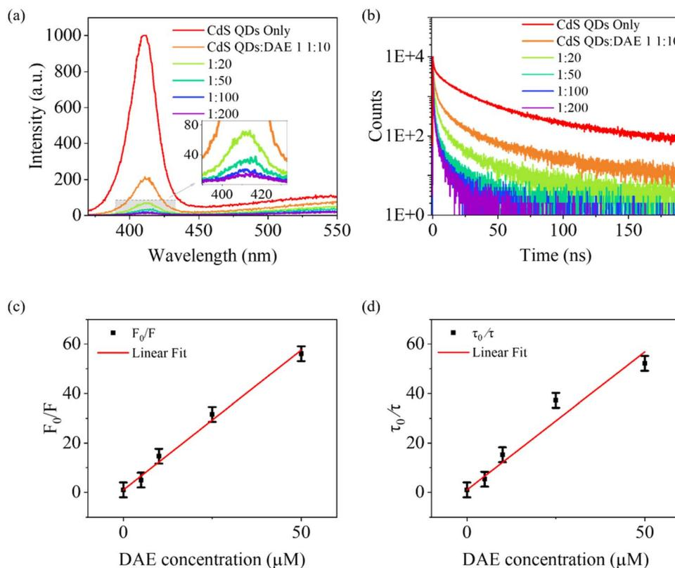
Fig. 2 Photoluminescence and quenching behavior of CdS QDs and **DAE 1**. (a) PL intensity quenching (insets show magnified time-resolved fluorescence quenching in the 390–430 nm range) and (b) PL lifetime of the CdS QD emission with and without **DAE 1** (relative concentrations of 10, 20, 50, 100 and 200) in toluene. Stern–Volmer plots and linear fits for (c) the PL intensity and (d) the PL lifetime quenching of CdS QDs.
