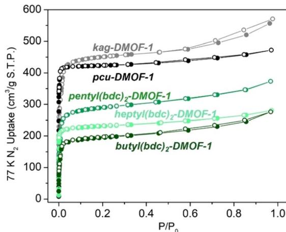
Fig. 6 N<sub>2</sub> sorption isotherms (77 K) of alkyl-tethered DMOFs in comparison with **pcu-DMOF-1** and **kag-DMOF-1**. Closed symbols represent adsorption and open symbols represent desorption.
