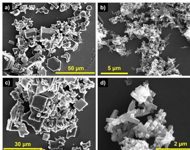
Fig. 8 Scanning Electron Microscopy (SEM) images of (a) **pentyl(bdc)<sub>2</sub>-DMOF-1**, (b) **pbdc-5a-DMOF-1**, (c) **heptyl(bdc)<sub>2</sub>-DMOF-1**, and (d) **pbdc-7a-DMOF-1**.
