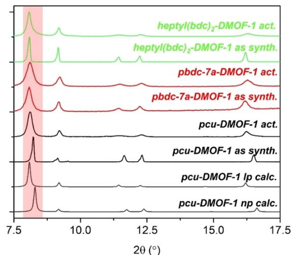
Fig. 7 PXRD patterns of as synthesized and activated DMOFs in comparison with **pcu-DMOF-1**. The red region highlights the (100) peak.
