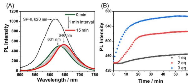
Fig. 6 (A) Time-dependent PL spectra of SP-II (assembled from  $\text{Pt-L}^1$  + 1.5 equiv. of  $\text{AgNO}_3$ ,  $\lambda_{\text{ex}} = 420$  nm) upon addition of  $\text{Fe}(\text{BF}_4)_2$  (3.0 equiv.) in  $\text{DMSO}/\text{H}_2\text{O}$  (9 : 1 v/v) at 293 K,  $\lambda_{\text{ex}} = 420$  nm. (B) Plots of PL intensity (at 650 nm) vs. times at different concentrations of  $\text{Fe}(\text{BF}_4)_2$ .
