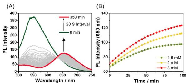
Fig. 5 (A) Time-dependent PL spectra of  $\text{Pt-L}^1$  (2.0 mM,  $\lambda_{\text{ex}} = 420$  nm) in the presence of  $\text{Fe}(\text{BF}_4)_2$  (1.5 equiv.) in  $\text{DMSO}/\text{H}_2\text{O}$  (9 : 1 v/v) at 293 K. (B) Plots for PL intensity at 650 nm vs. time at different concentrations of  $\text{Pt-L}^1$  (1.5–3.0 mM) in the presence of  $\text{Fe}(\text{BF}_4)_2$  (1.5 equiv.).
