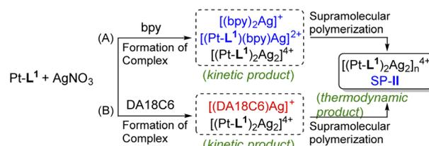
Scheme 2 Proposed formation mechanism of SP-II in the presence of either (A) bpy and Ag<sup>+</sup> or (B) DA18C6 and Ag<sup>+</sup> as secondary ligands.
