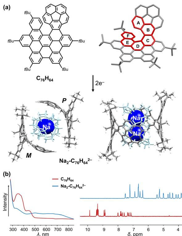
Fig. 1 (a) Structure of  $C_{76}H_{64}$  and chemical reduction to afford the dianion with  $Na^+$  ions in top and side views. (b) Comparison of UV-vis absorption and  $^1H$  NMR spectra of  $C_{76}H_{64}$  and its doubly-reduced product.<sup>88,89</sup>
