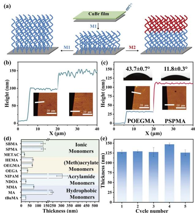
Fig. 3 (a) Schematic illustrating *in situ* chain growth of polymer brushes and preparation of diblock polymer brushes. The height analysis obtained by AFM of homo- (b) and block (c) polymer brushes. (d) Polymer brush thicknesses obtained by CuBr-mediated SI-CRP using CuBr<sub>0.1</sub> for 30 min with ionic, (meth)acrylate, acrylamide and hydrophobic monomers. (e) Reusability testing of CuBr<sub>0.1</sub> in CuBr-mediated SI-CRP.
