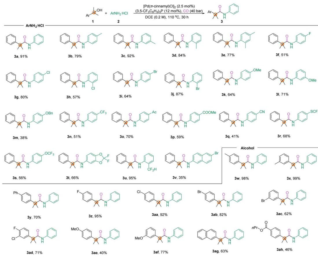
Scheme 2 Scope of aminocarbonylation toward amides with a quaternary carbon. Reaction conditions: alcohols (0.3 mmol, 1.5 equiv.),  $\text{ArNH}_2\text{HCl}$  (0.2 mmol, 1.0 equiv.),  $[Pd(\pi\text{-cinnamyl})Cl]_2$  (2.5 mmol%),  $(3,5\text{-CF}_3\text{C}_6\text{H}_3)_3\text{P}$  (12 mol%), CO (40 bar),  $110^\circ\text{C}$ , 30 h.
