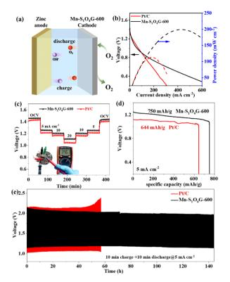
Fig. 4 (a) Schematic illustration of ZAB. (b) Discharging polarization and power density curves of Mn-S<sub>1</sub>O<sub>4</sub>G-600-based and Pt/C-based ZABs. (c) Galvanostatic discharge tests with various current densities for the  $Mn-S_1O_4G-600$ -based and Pt/C-based ZABs. (d) Specific discharging capacities at 5 mA cm<sup>-2</sup>. (e) The charge/discharge cycling performance of Mn-S<sub>1</sub>O<sub>4</sub>G-600-based and Pt/C-based ZABs at 5 mA  $cm^{-2}$
