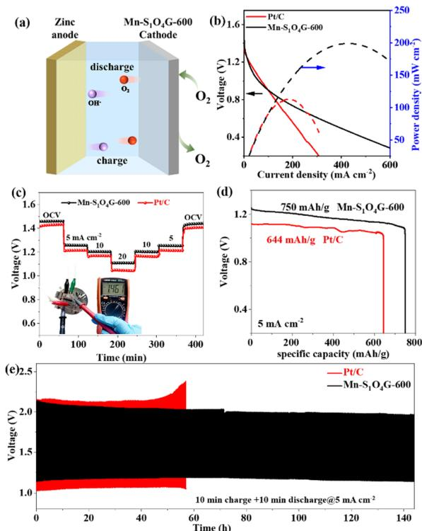
Fig. 4 (a) Schematic illustration of ZAB. (b) Discharging polarization and power density curves of Mn-S<sub>1</sub>O<sub>4</sub>G-600-based and Pt/C-based ZABs. (c) Galvanostatic discharge tests with various current densities for the Mn-S<sub>1</sub>O<sub>4</sub>G-600-based and Pt/C-based ZABs. (d) Specific discharging capacities at 5 mA cm<sup>-2</sup>. (e) The charge/discharge cycling performance of Mn-S<sub>1</sub>O<sub>4</sub>G-600-based and Pt/C-based ZABs at 5 mA cm<sup>-2</sup>.
