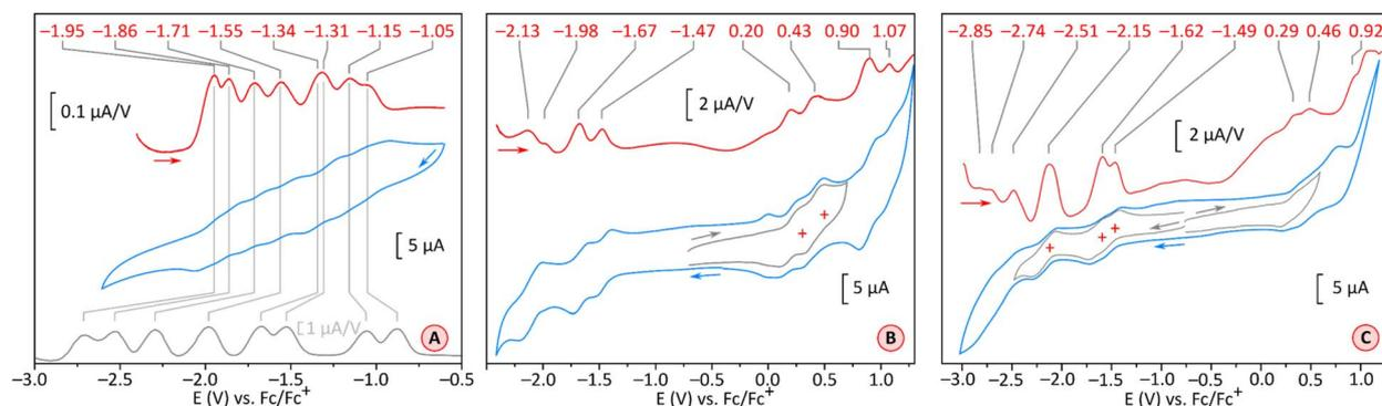
Fig. 4 Cyclic voltammograms (CV, blue traces) and differential pulse voltammograms (DPV, red traces) recorded for compound **2** (THF,  $[Bu_4N]PF_6$ , glassy-carbon electrode,  $100 \text{ mV s}^{-1}$ , panel (A)) and for compound **1** (in DCM,  $[Bu_4N]PF_6$ , glassy-carbon electrode,  $100 \text{ mV s}^{-1}$ , panel (B)); and in THF,  $[Bu_4N]PF_6$ , glassy-carbon electrode,  $100 \text{ mV s}^{-1}$ , panel (C)). The gray trace in panel (A) contains the reported DPV of TCTI.<sup>26</sup>
