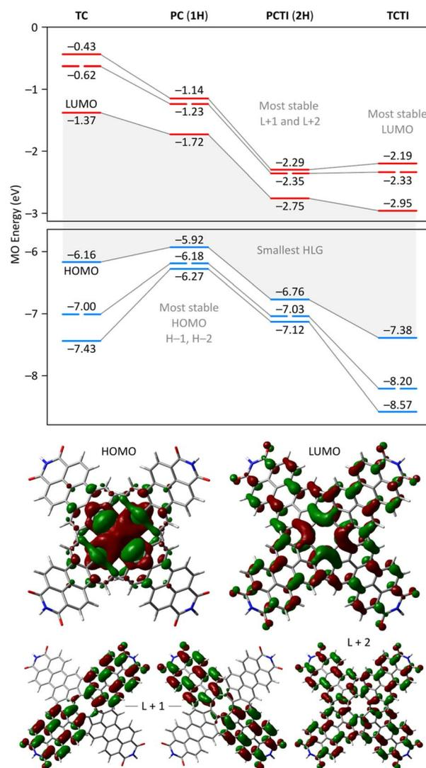
Fig. 8 Top: Kohn–Sham molecular orbital diagrams from the substituent-free tridecacyclenes and pentacosacyclenes **1H** and **2H** (GD3BJ-CAM-B3LYP/6-31G(d,p)). Gray lines connect the corresponding MO levels. Bottom: selected MO amplitudes for **2H**.
