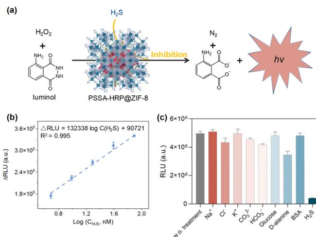
Fig. 6 (a) Schematic illustration of H<sub>2</sub>S sensing based on the PSSA-HRP@ZIF-8 composite combined with the luminol-H<sub>2</sub>O<sub>2</sub> system. (b) The linear range for H<sub>2</sub>S quantification. The concentration of HRP was set at 0.1 μg mL<sup>-1</sup>. (c) The selectivity of the proposed biosensor. The concentrations of H<sub>2</sub>S, BSA, and other interfering substances were 1 mM, 2 mM, and 10 mM, respectively.
