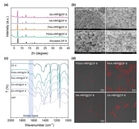
Fig. 2 PXRD patterns (a), SEM images (b), FT-IR spectra (c) and the merged CLSM images (d) of the PSSA-HRP@ZIF-8, PAA-HRP@ZIF-8, HA-HRP@ZIF-8, and SA-HRP@ZIF-8, where the polymer dosage for synthesis was kept at 0.5 mg for all biominerals.
