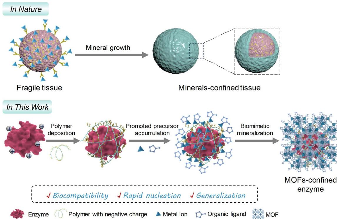
**Scheme 1** Schematic representation of the polymer deposition-mediated surface-charge reformation strategy for promoting biomineralization of MOFs on fragile enzymes with positive surface charges.
