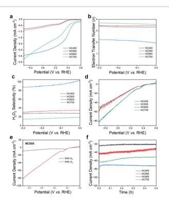
Fig. 2 (a) The RRDE LSV curves, (b) electron transfer number (n) and (c) the  $\rm H_2O_2$  selectivity of N-doped carbon catalysts calculated by RRDE. (d) The LSV curves of N-doped carbon catalysts, (e) the LSV curves of NC600 with and without O\_2, (f) the current density varied at electrolysis time at  $-0.35~\rm V_{RHE}$  of N-doped carbon catalysts.
