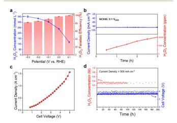
Fig. 3 The flow cell performance of NC600. (a)  $H_2O_2$  accumulated concentration and FE at varied potentials under a three-electrode system, (b) the current density and  $H_2O_2$  concentration at electrolysis time under a three-electrode system, (c) the LSV curve under a two-electrode system, (d) the  $H_2O_2$  instantaneous concentration and cell voltage at 500 mA cm $^{-2}$  varied with electrolysis time under a two-electrode system.
