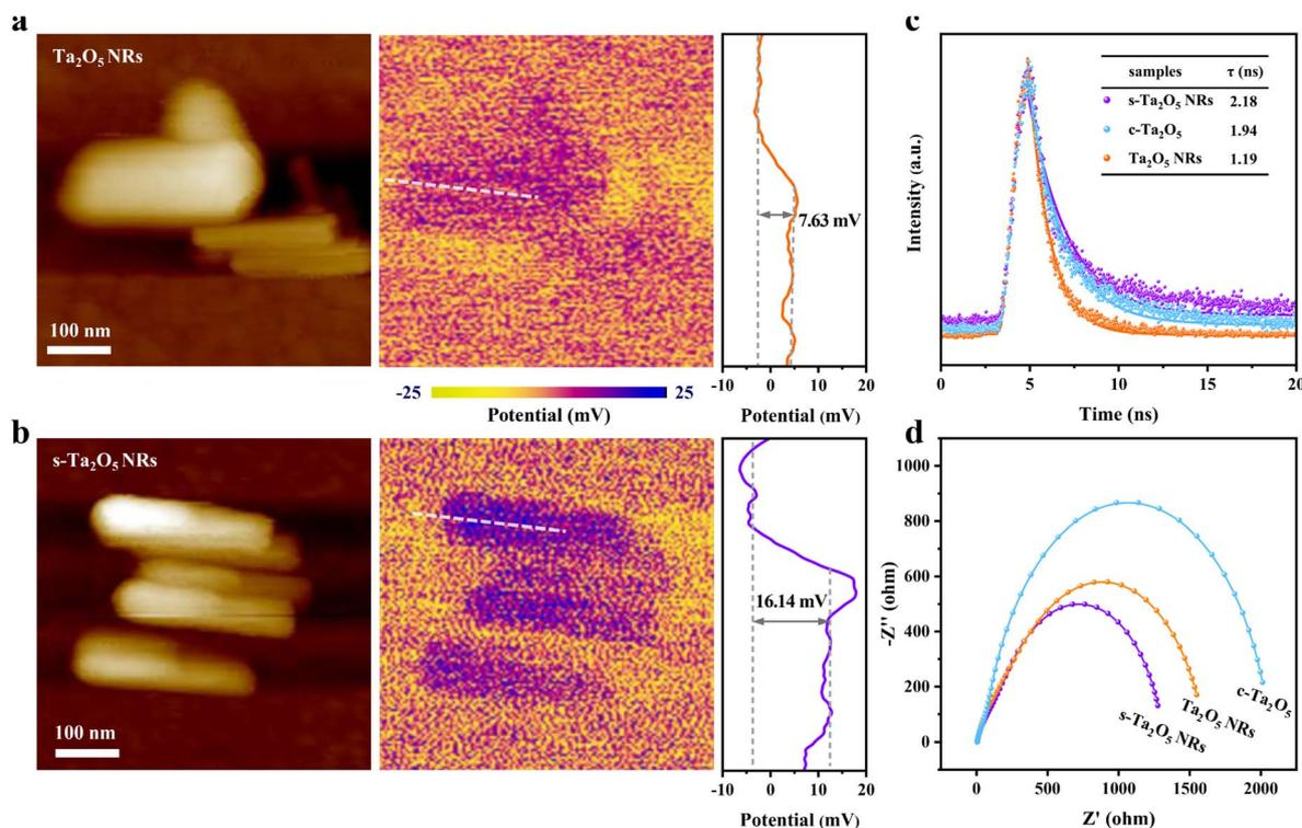
Fig. 4 The effect of tensile strain on charge transport in s- $\text{Ta}_2\text{O}_5$  NRs. Atomic force microscopy images (left) and the corresponding surface potentials measured with KPFM (right) of (a)  $\text{Ta}_2\text{O}_5$  NRs and (b) s- $\text{Ta}_2\text{O}_5$  NRs. (c) Time-resolved transient PL decay. (d) EIS spectra.
