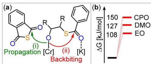
Fig. 4 (a) Model alkoxide intermediate comparing intermolecular propagation with PTA in pathway (i) with backbiting in pathway (ii). R = H (for EO), Me (for DMO),  $-C_3H_6-$  (for CPO). (b) Comparison of backbiting energies in pathway (b).
