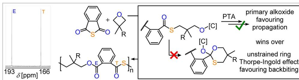
Fig. 5 Controlled PTA ROCOP with various 3,3'-geminally substituted oxetanes, revealing the importance of primary alkoxide formation. Zoom into the  $^{13}\text{C}$  NMR spectrum ( $\text{CDCl}_3$ ) of the PTA/3,3'-dimethyloxetane ROCOP product.
