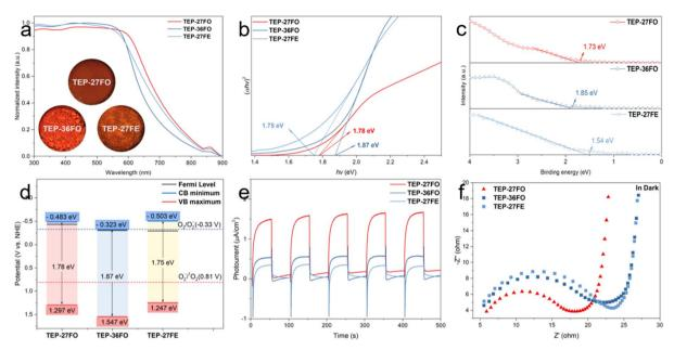
Fig. 2 (a) UV-vis DRS spectra of the TEP-X powders (inset: digital photograph). (b) Tauc plots with the band gaps. (c) VB-XPS spectra. (d) Energy band diagrams. (e) Transient photocurrent recorded under open-circuit conditions. (f) EIS Nyquist plots collected in the dark.
