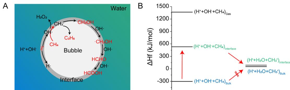
Fig. 5 (A) Proposed mechanism for the initiation of methane activation processes by water microbubbles. (B) Enthalpies of formation ( $kJ\ mol^{-1}$ ) in the gas-phase; on the surface of water microbubbles estimated by assuming that surface-bound ions are stabilized by half of the hydration enthalpies of gas-phase species; and in bulk water.
