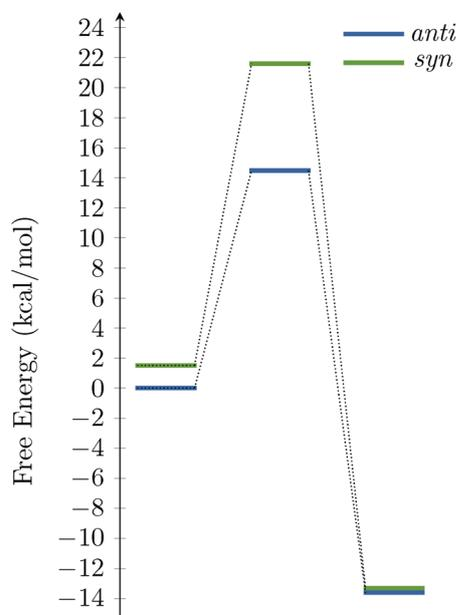
Fig. 5 Energies of the intermediate **IIaab** and HAT transition state (**TS2**) for *syn*- and *anti*-addition. Energies are: *anti*-**IIaab**, 0 kcal mol<sup>-1</sup>; *syn*-**IIaab**, 1.51 kcal mol<sup>-1</sup>; *anti*-**TS2**, 14.48 kcal mol<sup>-1</sup>; *syn*-**TS2**, 23.01 kcal mol<sup>-1</sup>; *anti*-**4aab**, -13.60 kcal mol<sup>-1</sup>; *syn*-**4aab**, -13.30 kcal mol<sup>-1</sup>.
