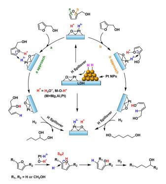
Fig. 4 Proposed mechanism for the ring-opening of FA over  $PtFe_x/DH$  catalyst.
