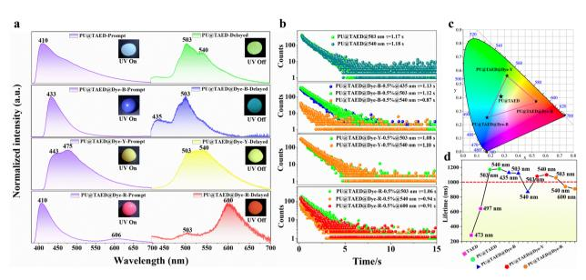
Fig. 3 (a) Steady-state prompt and delayed spectra of PU@TAED@Dye-B, PU@TAED@Dye-Y, and PU@TAED@Dye-R. Inset: corresponding photographs under and after removing the 365 nm UV lamp. (b-d) Phosphorescence lifetimes and CIE coordinate diagrams of PU@TAED@Dye-B, PU@TAED@Dye-B, PU@TAED@Dye-Y, and PU@TAED@Dye-R.
