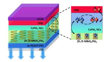
Fig. 14 Schematic representation, illustrating the spin-polarized charge injection and circularly polarised electroluminescence emission in spin-LEDs as demonstrated in the literature. The figure is reconstructed from ref. 62.
