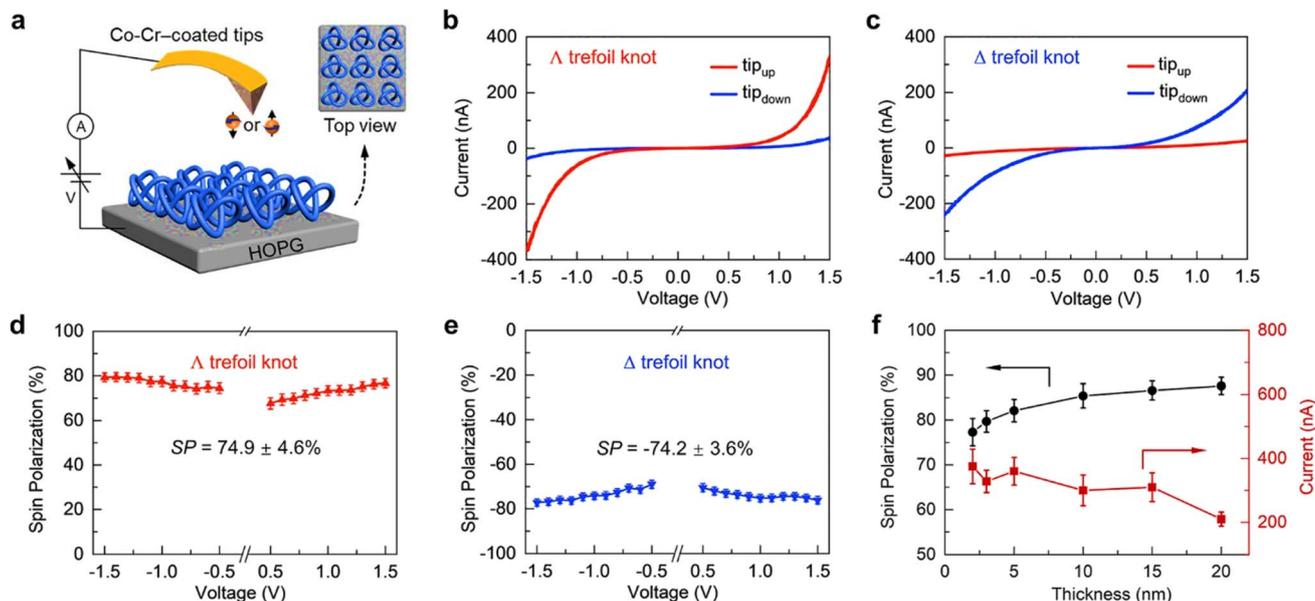
Fig. 9 (a) Representation of the mc-AFM setup. The averaged  $I$ - $V$  plots for  $\Lambda$  (b) and  $\Delta$  (c) molecular trefoil knots. The plot of spin polarization vs. applied voltages for  $\Lambda$  (d) and  $\Delta$  (e) knots. (f) Thickness-dependent SP% values and current intensities. Figures are adapted with permission from ref. 45 (copyright 2023, American Chemical Society).
