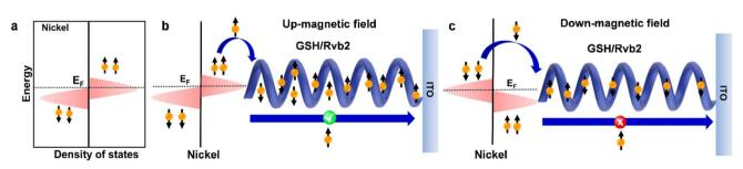
Fig. 4 Mechanistic model for spin-selective charge transport in Rvb2-based junctions. (a) Energy vs. density of states plot for the ferromagnetic Ni substrate in the absence of an applied magnetic field. (b and c) Proposed spin-selective charge transport in Ni/Rvb2/ITO junctions under spin-UP and spin-DOWN magnetic field conditions. Figures are adapted with permission from ref. 36 (copyright 2023, American Institute of Physics).
