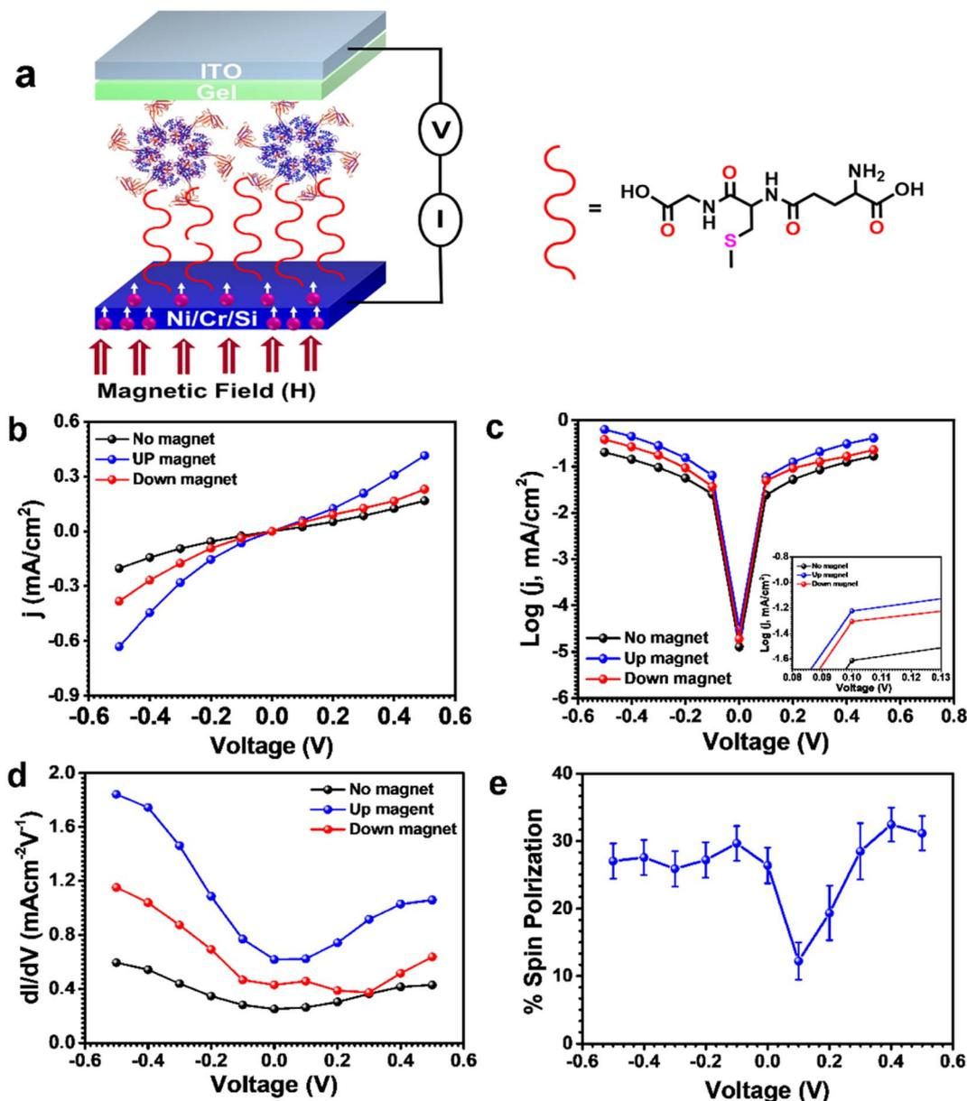
Fig. 3 Spin-selective charge transport in Rvb2-based biomolecular junctions. (a) Schematic illustration of the Ni/Rvb2/ITO biomolecular junction. (b)  $j$ - $V$  curves, (c) semilog curves and (d) derivative conductance curves of Ni/Rvb2/ITO biomolecular junctions in the absence and presence of an applied magnetic field. (e) Spin polarization as a function of applied bias. Figures are adapted with permission from ref. 36 (copyright 2023, American Institute of Physics).
