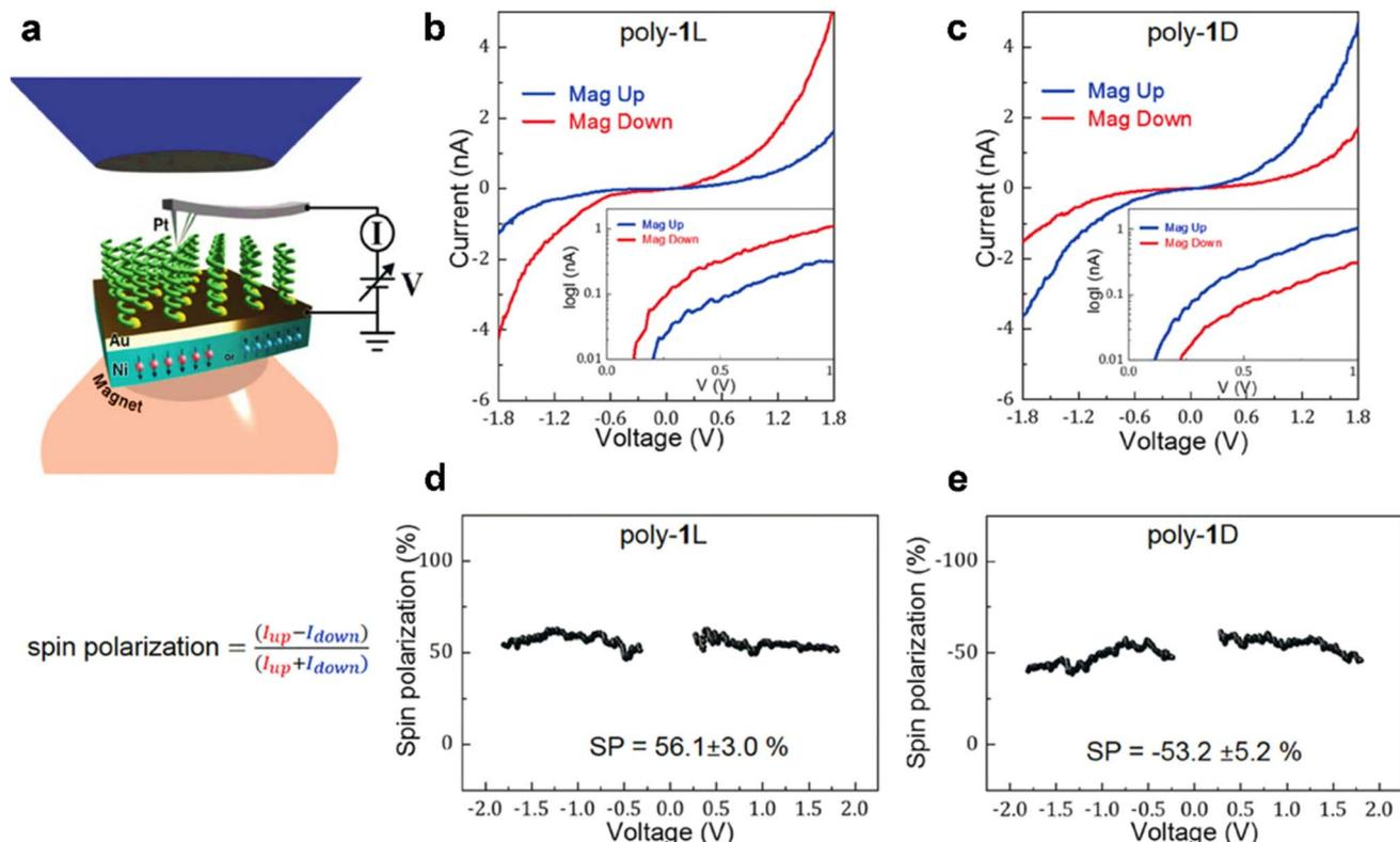
Fig. 7 (a) Scheme of the mc-AFM setup. (b and c) Averaged  $I-V$  plots for L and D polymers, respectively. (d and e) The spin polarization vs. voltage plots for L and D polymers, respectively. Figures are adapted with permission from ref. 40 (copyright 2020, Wiley).
