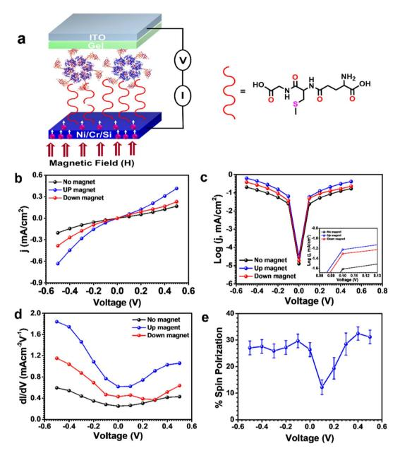
Fig. 3 Spin-selective charge transport in Rvb2-based biomolecular junctions. (a) Schematic illustration of the Ni/Rvb2/ITO biomolecular junction. (b) j-V curves, (c) semilog curves and (d) derivative conductance curves of Ni/Rvb2/ITO biomolecular junctions in the absence and presence of an applied magnetic field. (e) Spin polarization as a function of applied bias. Figures are adapted with permission from ref. 36 (copyright 2023, American Institute of Physics).
