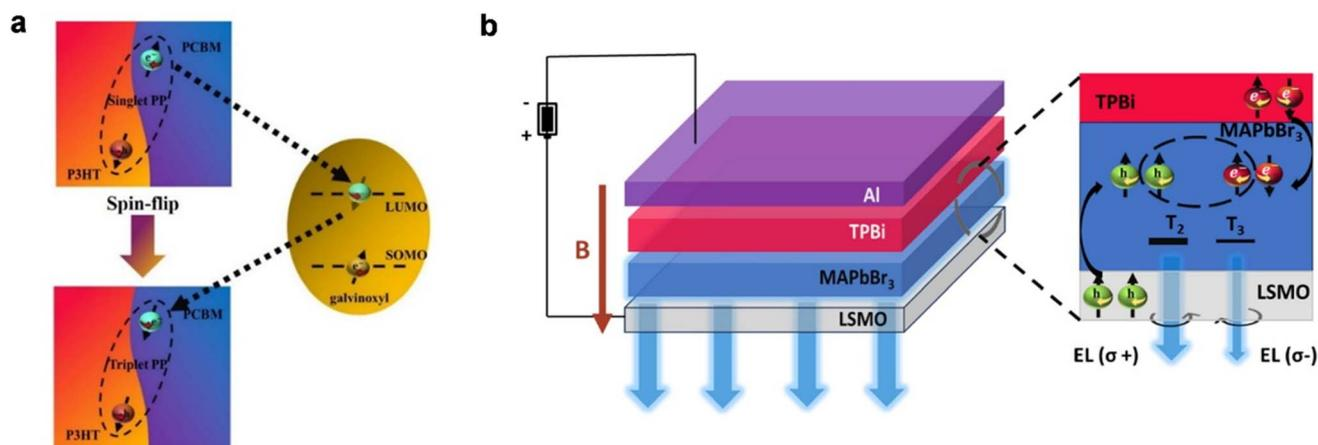
Fig. 13 (a). Schematic representation of the spin-flipping mechanism *via* galvinoxyl radicals. (b). Schematic representation of the spin-LED device architecture consisting of a half-metal LSMO anode, MAPbBr<sub>3</sub> light emitting layer, and TPBi molecule thin film as the electron transport layer covered with an Al cathode. Figure (a) is reconstructed from ref. 54. Figure (b) is adapted with permission from ref. 60.
