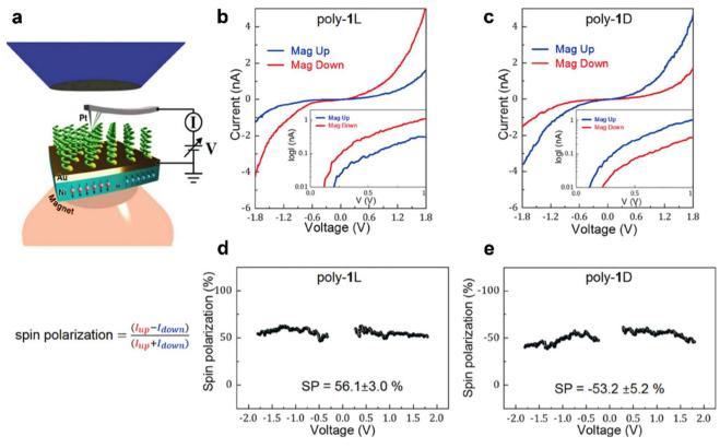
Fig. 7 (a) Scheme of the mc-AFM setup. (b and c) Averaged *I–V* plots for L and D polymers, respectively. (d and e) The spin polarization *vs.* voltage plots for L and D polymers, respectively. Figures are adapted with permission from ref. 40 (copyright 2020, Wiley).
