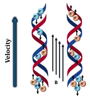
Scheme 1 Schematic representation of the CISS effect where the electron transfer process happens through a chiral potential that facilitates spin-selective electron transmission.
