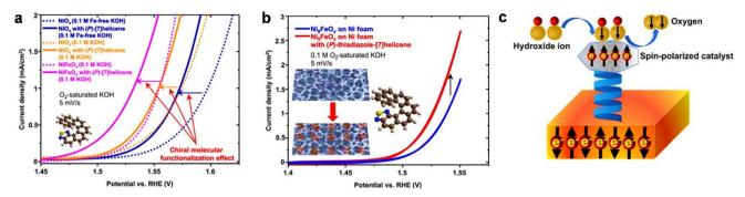
Fig. 19 Current density vs. applied potential plots (a) to check the effect of chiral modification on NiO<sub>x</sub> islands in Fe-free KOH, NiO<sub>x</sub> islands in unpurified KOH, and NiFeO<sub>x</sub> islands in unpurified KOH and (b) to check the chiral molecular functionalization enhancement at Ni<sub>x</sub>FeO<sub>x</sub> deposited on Ni foam. (c) Proposed mechanism of the OER. Figures are adapted with permission from ref. 76 (copyright @2022, Nature Communications).
