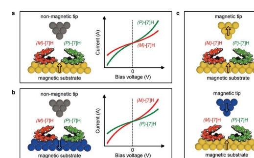
Fig. 1 (a and b) Demonstrating the magneto-chiral electron tunneling on the ferromagnetic electrode for heptahelicene enantiomers. (c) Measurements of STM conductance with a magnetic STM tip on a ferromagnetic substrate. Figures are adapted with permission from ref. 31 (copyright 2023, Wiley).
