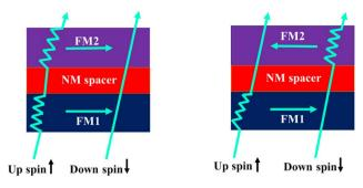
Fig. 10 Schematic representation of a spin-valve structure demonstrating spin-dependent scattering at the two ferromagnetic electrodes in both parallel and antiparallel alignments as shown in the literature. The figure is reconstructed from ref. 47.
