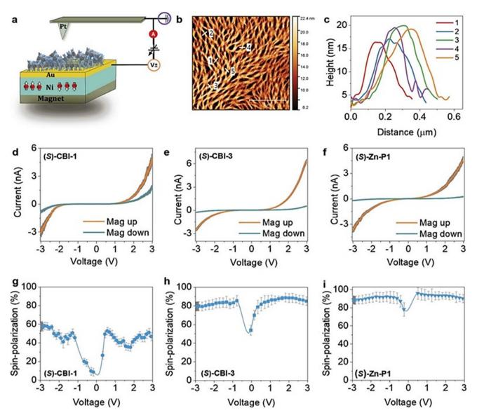
Fig. 5 (a) Representation of the mc-AFM setup. (b and c) AFM image of the supramolecular nanofibers and AFM height profiles. (d-f) The averaged I-V plots for different samples showing the Ni film magnetized with the north pole pointing up (orange) or down (cyan). (g-i) The plot of SP% vs. voltage for different samples. Figures are adapted with permission from ref. 39 (copyright 2020, Wiley).
