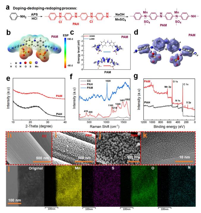
Fig. 1 Synthesis, theoretical modeling and characterization of PANI-based electrodes. (a) Synthesis of H<sup>+</sup>-doped PANI (PAH) and Mn<sup>2+</sup>-doped PANI (PAM); (b) electrostatic potential (ESP) distribution, (c) calculated energy levels and (d)  $\pi$ -electron localization function image of the optimized PAM monomer; (e) XRD patterns, (f) Raman and (g) XPS spectra of PAH and PAM; SEM images of (h) carbon cloth, (i) PAH and (j) PAM; (k) TEM and (l) mapping images of PAM.
