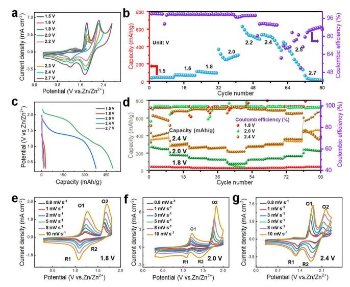
Fig. 5 Electrochemical behavior of Zn//PAM cells in different voltage ranges. (a) CV curves in the voltage range from 1.5 V to 2.7 V at a scan rate of 10 mV s<sup>-1</sup>, (b) capacity and coulombic efficiency at different voltages at a current density of 0.5 A g<sup>-1</sup>, (c) GCD curves at a current density of 0.5 A g<sup>-1</sup>; (d) rate capability in the voltage range from 1.8 V to 2.4 V; (e–g) CV curves of cells at different scan rates.
