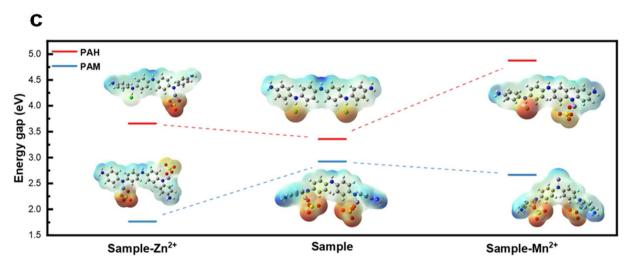
Fig. 7 Schematic diagram of the interactive dual energy storage mechanism of PAM. (a) Mechanism I: reversible doping mechanism of  $Mn^{2+}$  along with  $H^+$  and  $Zn^+$  into the conjugated backbone. (b) Mechanism II: dissolution–deposition storage mechanism of  $Mn^{2+}$  on the cathode surface. (c) The plot of energy gap variation for PAH and PAM sample materials doped with  $ZnSO_4$  and  $MnSO_4$  electrolytes.
