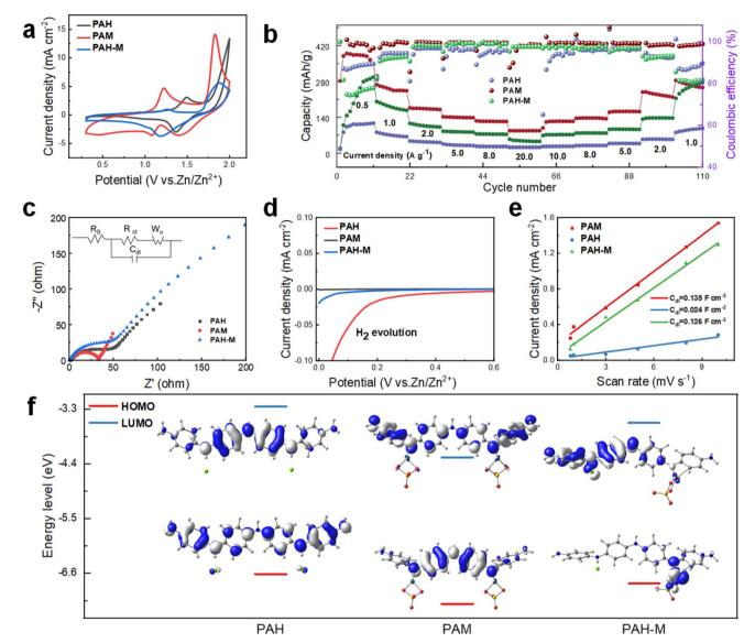
Fig. 2 Electrochemical performance of PAH, PAM and PAH-M electrodes in 2 M ZnSO<sub>4</sub> electrolyte. (a) CV curves, (b) rate capability, (c) EIS curves, (d) LSV curves, and (e) double layer capacitance linear fitting diagram; (f) chemical structures and calculated energy levels of the optimized PAH, PAM and PAH-M monomers.
