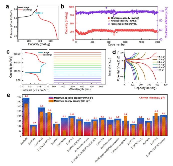
Fig. 4 Electrochemical performance of Zn//PAM cells. (a) Self-discharge behavior after resting for 24 h, (b) the capacity retention after 2000 cycles at a current density of  $1 \text{ A g}^{-1}$ , (c) in situ UV-vis curves of the  $2 \text{ M ZnSO}_4$  electrolyte during a GCD cycle, (d) GCD curves at different current densities of  $1-10 \text{ A g}^{-1}$ , and (e) the capacity and energy density comparison among reported PANI-based AZIBs.
