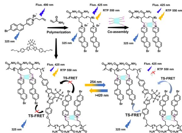
Fig. 7 Schematic illustration of a solid supramolecular polymer with tunable ultra-strong white-light emission constructed using bromonaphthylpyridinium polymerization, sulfobutylether- $\beta$ -CD, and a diarylethene derivative. This figure has been adapted from ref. 36 with permission from Wiley-VCH GmbH, copyright 2022.
