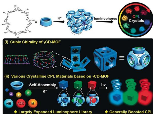
Fig. 19 A crystalline CPL material constructed using  $\gamma$ -CD-MOFs and achiral luminescent groups with different charges and sizes. This figure has been adapted from ref. 70 with permission from Wiley-VCH GmbH, copyright 2020.
