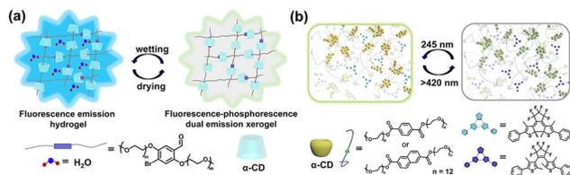
Fig. 12 (a) Schematic illustration of a CD-based polypseudorotaxane xerogel exhibiting RTP and water-stimulated switchable white-light emission features. This figure has been adapted from ref. 54 with permission from Wiley-VCH GmbH, copyright 2019. (b) Schematic illustration of photoreversible multicolor RTP supramolecular pseudopolyrotaxanes. This figure has been adapted from ref. 55 with permission from Wiley-VCH GmbH, copyright 2022.
