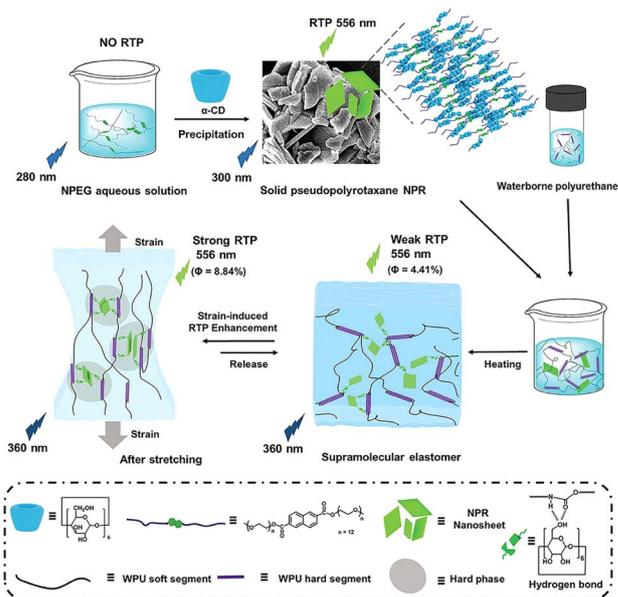
Fig. 13 Schematic illustration of  $\alpha$ -CD pseudopolyrotaxane elastomers exhibiting reversible mechanical stretching-induced RTP enhancement behavior. This figure has been reproduced from ref. 57 with permission from the authors, copyright 2024.
