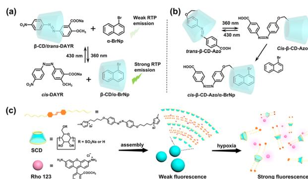
Fig. 8 (a) The reversible assembly mode based on the  $\beta$ -CD/DAYR/ $\alpha$ -BrNp ternary system for photocontrolled RTP emission. (b) Photo-response phenomenon of pseudorotaxane  $\beta$ -CD-Azo and the co-assembly with  $\alpha$ -BrNp. (c) Schematic illustration of a non-covalent hypoxia-responsive ternary fluorescent supramolecular probe. This figure has been adapted from ref. 42 with permission from American Chemical Society, copyright 2022.
