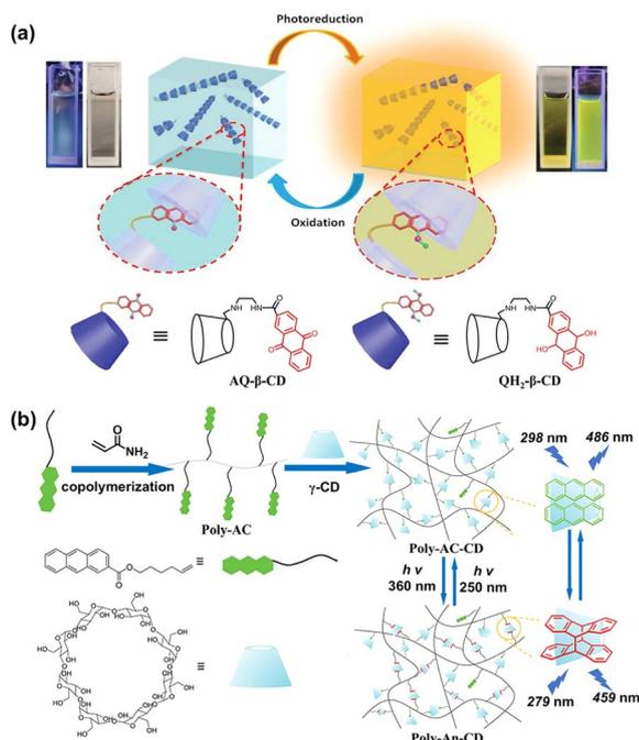
Fig. 9 (a) Photoreduction and oxidation luminescence properties of AQ- $\beta$ -CD-based supramolecular non-covalent polymers in aqueous solution. This figure has been adapted from ref. 43 with permission from the authors, copyright 2020. (b) Schematic diagram of dynamic self-assembly of  $\gamma$ -CD and anthracene-acrylamide copolymers and its reversible photo-responsiveness. This figure has been adapted from ref. 44 with permission from Wiley-VCH GmbH, copyright 2021.
