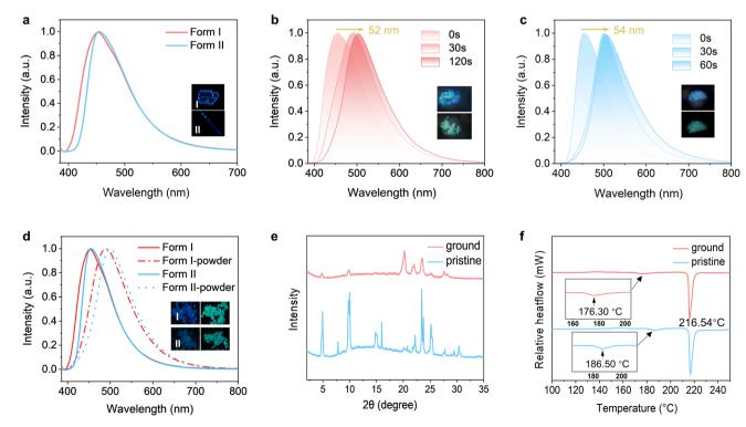
Fig. 3 (a-d) PL spectra and luminescent photographs of: Form I and Form II (a), Form I under 365 nm UV light irradiation (b), Form II under 365 nm UV light irradiation (c), and ground Form I and Form II (d). (e) PXRD patterns of Form I and the ground samples. (f) DSC curves of Form I and the ground samples
