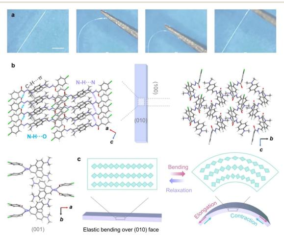
Fig. 4 (a) Elastic bending processes of the Form II crystals along the (010) facet. (b) Molecular packing and intermolecular interactions of Form II. (c) Schematic diagram showing the changes of the molecules inside the crystal during elastic bending. The scale bar is 200 μm.
