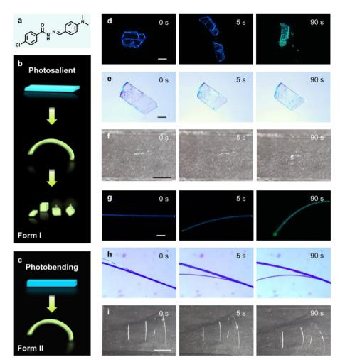
Fig. 1 (a) Chemical formula of CDBB. (b and c) Schematic diagrams of the photosalient and photoinduced bending process. (d-f) Images of the photosalient crystals under visible and UV light: 365 nm (d), 425 nm (e), and natural light (f). (q-i) Images of the photoinduced bending crystals under visible and UV light: 365 nm (g), 425 nm (h), and natural light (i). The scale bar is 200 µm (d, e, g and h) and 1 cm (f and i).
