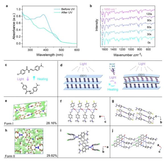
Fig. 2 (a) Absorption spectra of pristine and irradiated samples of Form I. (b) FTIR spectra of irradiated Form I taken at 30 s time intervals. (c) Schematic diagram of CDBB before and after isomerization. (d) Schematic of the mechanism for the photoinduced bending of the Form I and Form II crystals. (e–g) Fractional free volume and intermolecular interactions of Form I. (h–j) Fractional free volume and intermolecular interactions of Form II.
