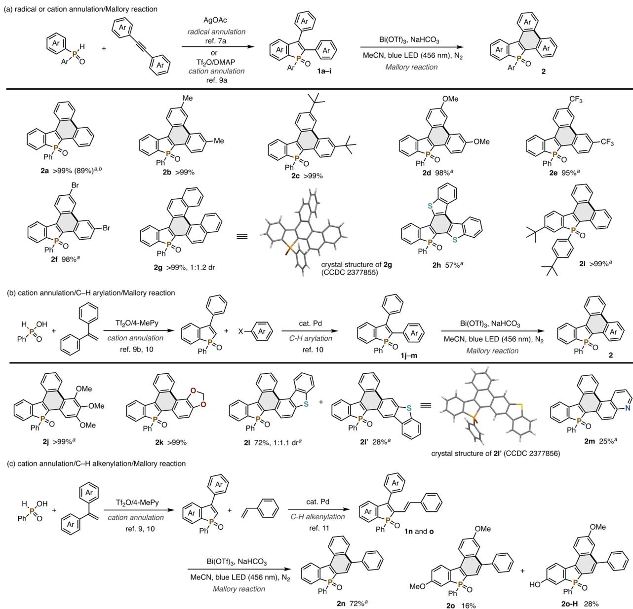
**Scheme 2** Products of the  $\text{Bi}(\text{OTf})_3$ -assisted dehydrogenative Mallory reaction of phosphole derivatives **1**. Isolated yields are shown. Conditions of the Mallory reaction: **1** (0.030–0.11 mmol),  $\text{Bi}(\text{OTf})_3$  (1.0 equiv.),  $\text{NaHCO}_3$  (1.0 equiv.), MeCN (1.0 mL), blue LED (456 nm, 40 W), ambient temperature (40–50 °C under light irradiation), 22 h,  $\text{N}_2$ . <sup>a</sup>With two LEDs (40 W × 2). <sup>b</sup>On a 1.0 mmol scale.
