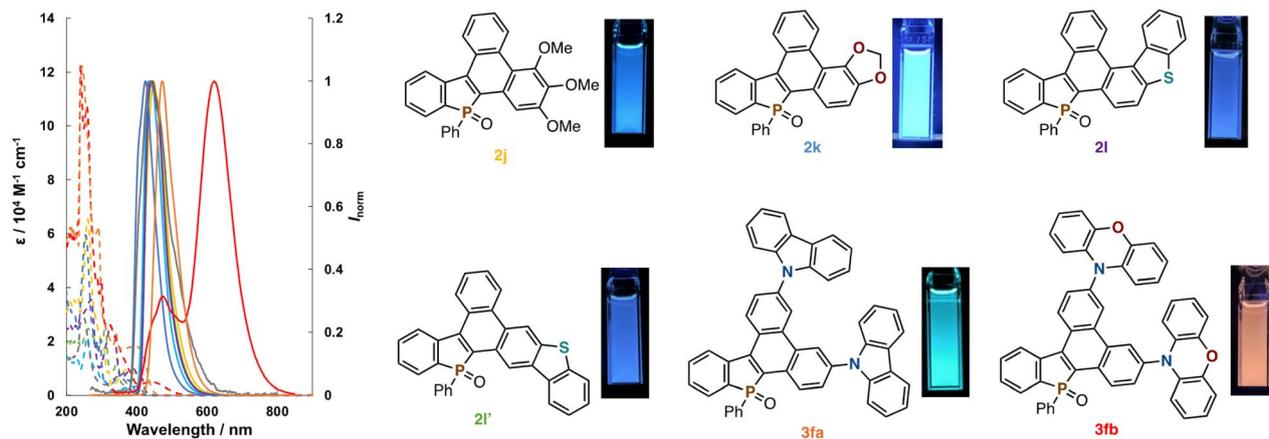
Fig. 1 UV-vis absorption (dashed lines) and fluorescence spectra (solid lines) of **1a**, **2a**, **2j**, **2k**, **2l**, **2l'**, **3fa**, and **3fb** in  $\text{CHCl}_3$  ( $1.0 \times 10^{-5}$  M), and fluorescence images of **2j**, **2k**, **2l**, **2l'**, **3fa**, and **3fb**.
