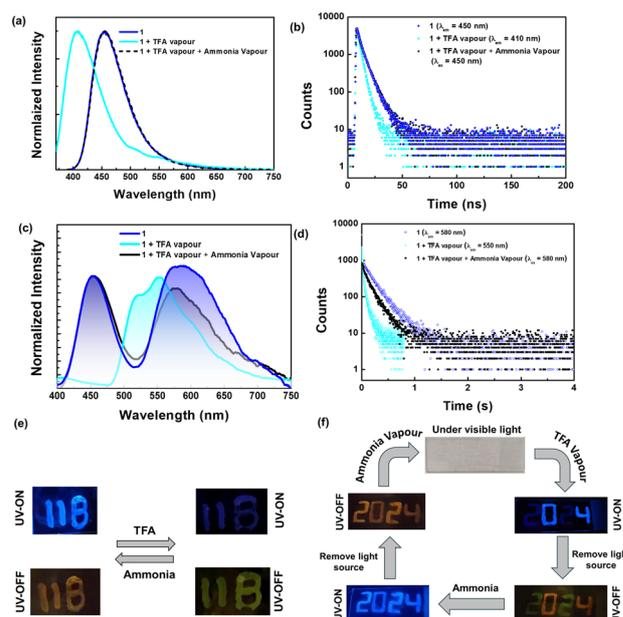
Fig. 8 (a) Fluorescence spectra and (c) phosphorescence spectra [smoothened up to 50 pt for clarity, unsmoothed spectra in ESI Fig. S66d†] (b and d) time-resolved decay for **1** doped in the PMMA film (1 wt%). Photographs illustrating (e) pH-sensitive emission features of the doped film (1 wt% in PMMA) and (f) the anti-counterfeiting application of the **1** film (1 wt% in PMMA) by exploring pH-sensitive emission features.
