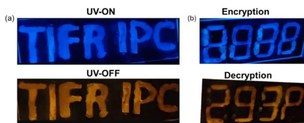
Fig. 7 Digital photographs of (a) writing done with ink made from a mixture of PMMA and **1** (1 wt%) under UV on and off conditions. (b) Anti-counterfeiting demonstration using ink made from a mixture of PMMA and **1** (1 wt% and 50 wt%) compound **1** utilizing single molecular pRTP emission features of **1**.
