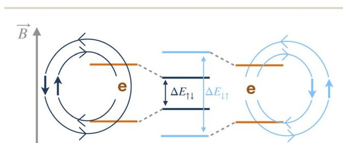
Fig. 1 Two different pair orientations of nuclear spins,  $|\downarrow\uparrow\rangle$  and  $|\uparrow\downarrow\rangle$ , interacting with an electron are shown on the left and right, respectively. Their different orientations and distances from the electron rescale the Zeeman energy, as shown in the middle of the diagram.
