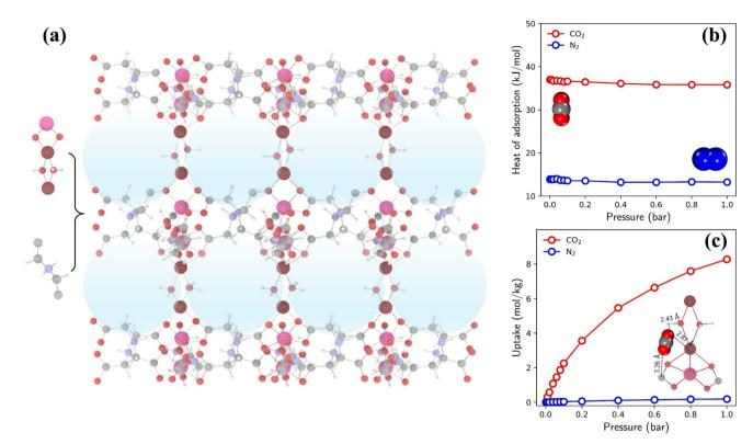
Fig. 6 (a) Structure of a top-performing MOF (assembled from metal vertice m160 and organic edge o323) for  $CO_2$  capture, with blue spheres indicating the largest cavities. (b) Heats of  $CO_2$  and  $N_2$  adsorption. (c) Isotherms of  $CO_2$  and  $N_2$  adsorption, with a simulation snapshot highlighting the preferential adsorption site of  $CO_2$ .
