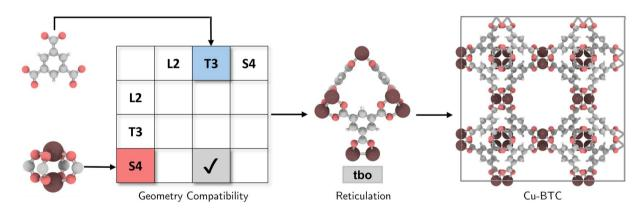
Fig. 2 Selection of a compatible topology for the assembly of Cu paddlewheel ( $Cu_2O_8$ ) and 1,3,5-benzene tricarboxylate (BTC), followed by reticulation into a 'reticular ideal' **tbo** topology, constructing Cu-BTC.
