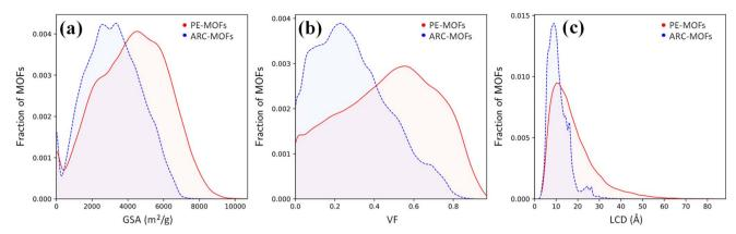
Fig. 3 Distributions of (a) GSA, (b) VF and (c) LCD in 94 823 PE-MOFs (red) and 279 010 ARC-MOFs (blue). 14
