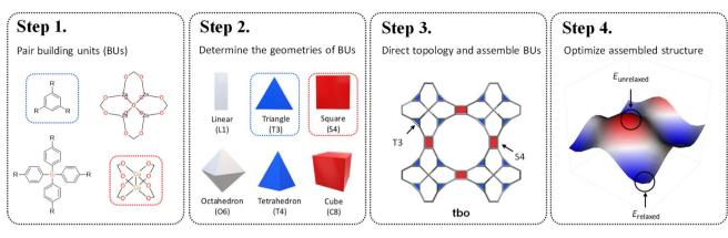
**Scheme 1** Topological structure prediction with precision engineering. Step 1: pair building units; Step 2: determine the geometries of building units; Step 3: direct topology and assemble building units; Step 4: optimize assembled structure.
