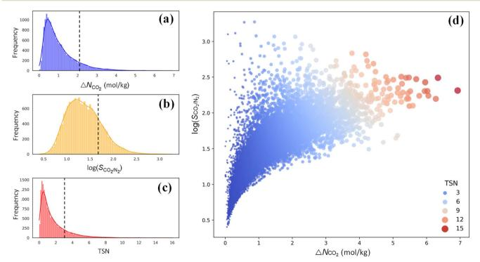
Fig. 5 Performance of 17 173 PE-MOFs for CO<sub>2</sub> capture. (a–c) Distributions of  $\Delta N_{\text{CO}_2}$ ,  $\log(S_{\text{CO}_2/N_2})$  and TSN in 17 173 PE-MOFs. The dashed line denotes the performance of zeolite-13X as a benchmark.<sup>38</sup> (d)  $\log(S_{\text{CO}_2/N_2})$  versus  $\Delta N_{\text{CO}_2}$ , with the color-coding based on TSN.
