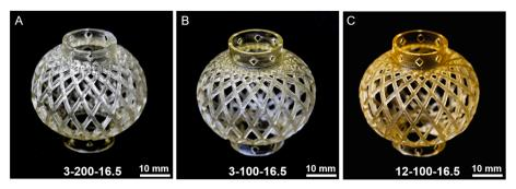
Fig. 7 3D printed Chinese lantern models using three types of macroCTA with pendant CTA groups at 16.5 wt% loading. (A) 3-200; (B) 3-100; (C) 12-100. The objects were 3D printed at layer cure time of 40 s with a layer thickness of 100  $\mu$ m with a molar ratio of [AA]/[PEGDA] = 4/1 in resins.
