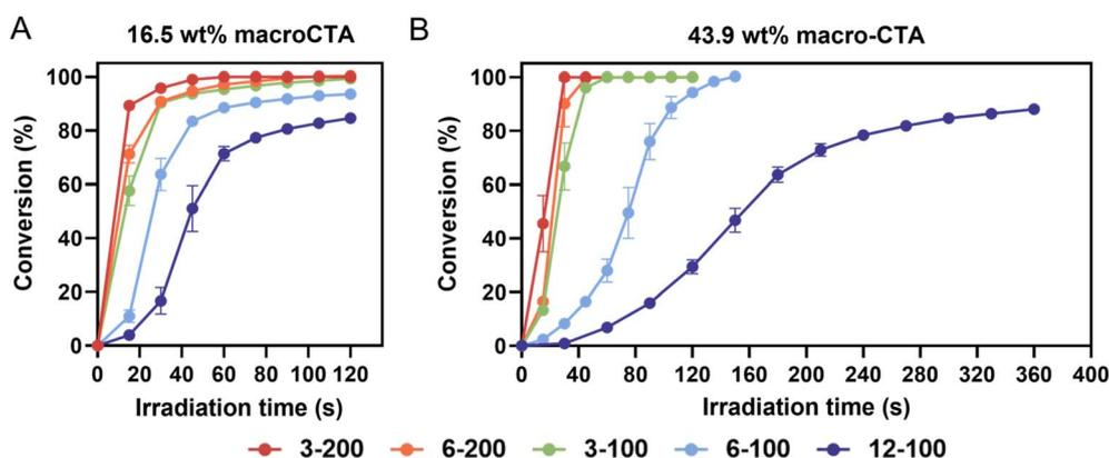
Fig. 2 Polymerization kinetics of resins with different macroCTAs and varied mass loading. (A) Resins with 16.5 wt% of macroCTAs (3-200, 6-200, 3-100, 6-100, and 12-100); (B) resins with 43.9 wt% of macroCTAs (3-200, 6-200, 3-100, and 12-100). The kinetics experiments were performed in triplicate. Error bars indicate standard deviation in triplicate measurements. Some error bars fall within the size of the markers.
