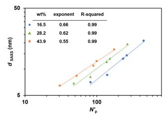
Fig. 5 Power law regression lines for domain spacing of 3D printed PIMS materials. log–log plot of domain spacing ( $d_{SAXS}$ ) as a function of normalized total degree of polymerization per CTA group ( $N'_p$ ).  $d_{SAXS}$  was determined from SAXS.  $N'_p$  was normalized based on a common monomer reference volume (118 Å<sup>3</sup>). Scaling exponents and R-squared values are shown in the inset table.
