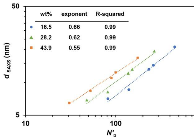
Fig. 5 Power law regression lines for domain spacing of 3D printed PIMS materials. log–log plot of domain spacing ( $d_{\text{SAXS}}$ ) as a function of normalized total degree of polymerization per CTA group ( $N'_p$ ).  $d_{\text{SAXS}}$  was determined from SAXS.  $N'_p$  was normalized based on a common monomer reference volume (118 Å<sup>3</sup>). Scaling exponents and  $R$ -squared values are shown in the inset table.
