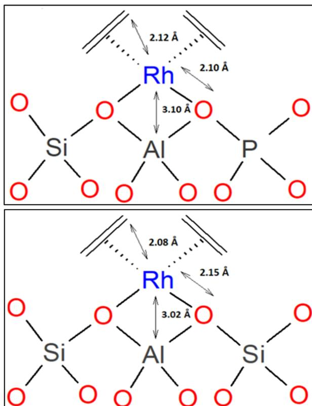
Scheme 1 Structural models of rhodium diethene complex on SAPO-37 (top)<sup>61</sup> and rhodium diethene complex on DAY zeolite (bottom)<sup>60</sup> determined by EXAFS spectroscopy. Reproduced from ref. 61 with permission from the American Chemical Society, Copyright 2021.
