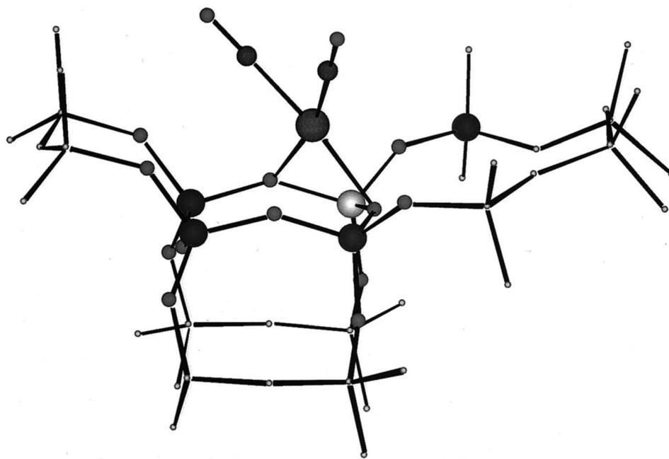
Fig. 3 Location of rhodium dicarbonyl complex at a four-ring of dealuminated HY zeolite. The atoms included in the isolated DFT cluster model are shown as circles, with the rhodium atom in the upper center shown with two carbonyl ligands. Below that, in the four-ring, are three silicon atoms and one aluminum atom.<sup>59</sup> The dangling bonds of the cluster model are capped by hydrogen atoms. Reproduced from ref. 59 with permission from the American Chemical Society. Copyright 2000.
