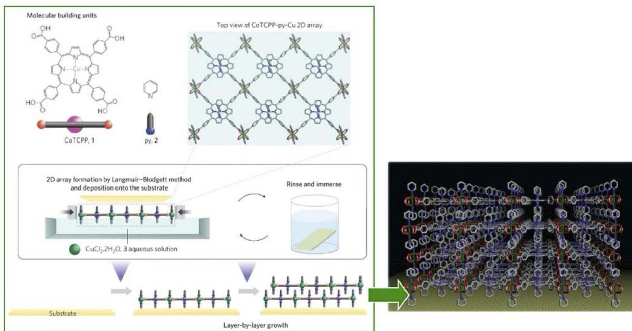
Fig. 16 MOF monolayers obtained by developing 5,10,15,20-tetrakis(4-carboxyphenyl)porphyrinato-cobalt(II) and pyridine on a solution of  $\text{CuCl}_2 \cdot 2\text{H}_2\text{O}$  in chloroform/methanol that is multilayered by a sequential LbL stacking procedure. Reprinted with permission from ref. 95 Copyright 2010 Springer-Nature.
