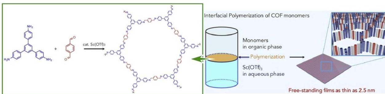
Fig. 17 COFs with imine bonding obtained by interfacial polymerization of 1,3,5-tris(4-aminophenyl)benzene and terephthalaldehyde as monomers using  $\text{Sc}(\text{OTf})_3$ , a Lewis acid catalyst, resulting in nanoarchitectonics of a continuous COF film at the interface. Reprinted with permission from ref. 97 Copyright 2018 Elsevier.
