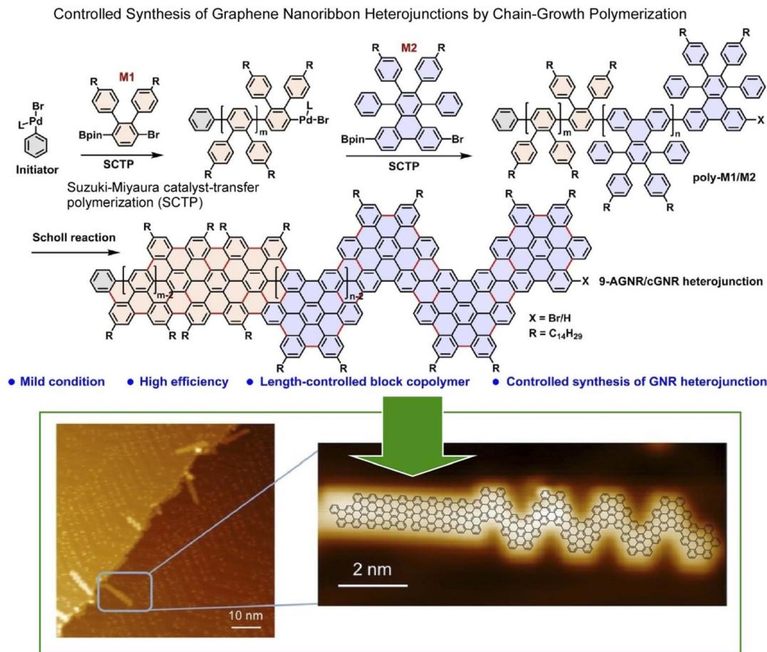
Fig. 2 On-surface synthesis of graphene nanoribbon heterojunctions from block polyphenylene precursors by chain-growth polymerization: chemical reaction (top) and molecular-level imaging by *in situ* scanning tunnelling microscopy (bottom). Reproduced under terms of the CC-BY license from ref. 51, 2023 Wiley-VCH.
