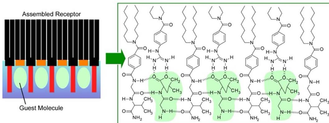
Fig. 7 Associated receptor at the air–water interface: an equimolar mixed monolayer of a dioctadecylglycylglycinamide amphiphile and a functional amphiphile with guanidinium groups for the optimal recognition structure of a water-soluble dipeptide (left: guest molecules and right: green labels).
