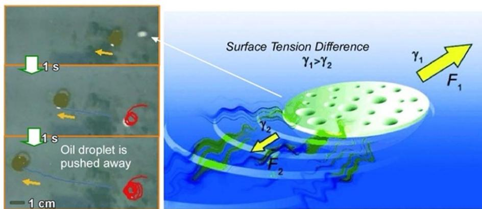
Fig. 19 Polymer capsule motor running on a liquid surface upon asymmetric changes in the surface tension of the surrounding liquid due to the Marangoni effect. Photos on the left side demonstrate oil droplet pushing by the capsule motor. Reprinted with permission from ref. 101 Copyright 2011 Wiley-VCH.
