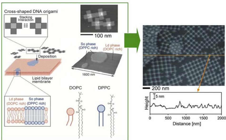
Fig. 22 Environment-dependent self-assembly of DNA origami lattices on phase-separated lipid membranes: DNA origami on the liquid disordered phase formed 2D lattices, while DNA origami on the solid ordered phase formed aggregates (right AFM image of DNA origami on a lipid membrane). Reprinted with permission from ref. 109 Copyright 2018 Wiley-VCH.
