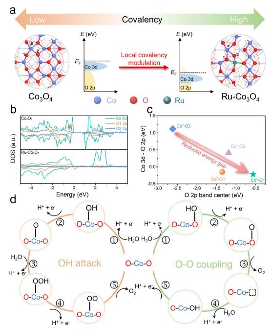
Fig. 1 Electronic structures and OER pathways. (a) Structures and schematic energy bands of  $Co_3O_4$  and  $Ru-Co_3O_4$  (the corresponding structure is shown in Fig. S5a†). (b) Computed DOS of Co 3d and O 2p for  $Co_3O_4$  and  $Ru-Co_3O_4$ . (c) Energy gap between Co 3d and O 2p *versus* the O 2p band center for  $Co_3O_4$  and  $Ru-Co_3O_4$ . (d) Proposed transformation of the OER mechanism from the AEM to LOM after the doping of Ru.
