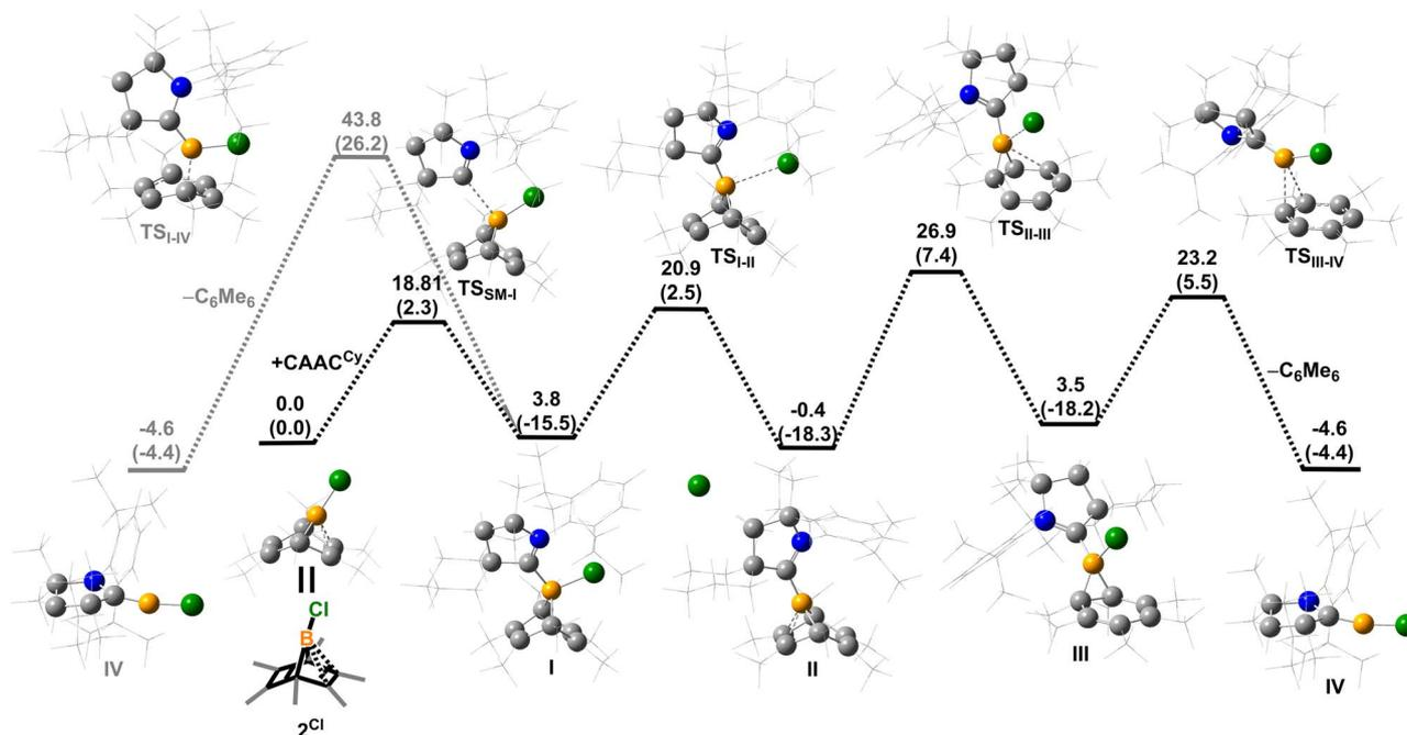
Fig. 3 Energy profiles calculated for the reaction from  $\text{SM}$  to  $\text{IV}$  and from  $\text{I}$  to  $\text{IV}$ . The relative Gibbs free energies (calculated at 298 K) and electronic energies (in parentheses) are given in kcal mol<sup>-1</sup> (in scale). ( $\omega\text{B97xD}/6\text{-}311\text{G}^{**}/\omega\text{B97M-V}/\text{def2-QZVPP}$  level of theory).
