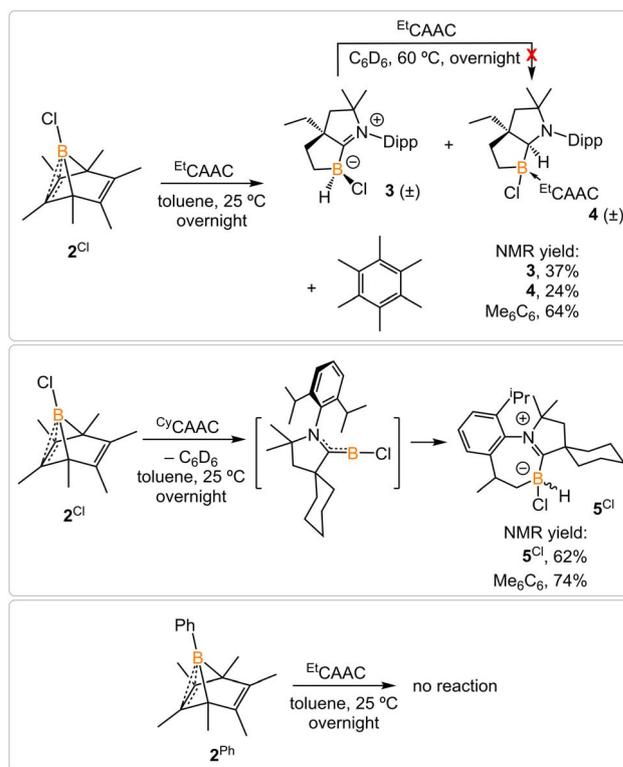
Scheme 2 Treatment of **2<sup>Cl</sup>** with  $EtCAAC$  and  $CyCAAC$  and attempt to generate phenylborylene.
