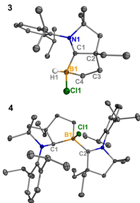
Fig. 2 Molecular structures of **3** and **4** in the solid-state. Hydrogen atoms, except for the one connected to B1, have been omitted for clarity. Thermal ellipsoids are drawn at the 50% probability level.
