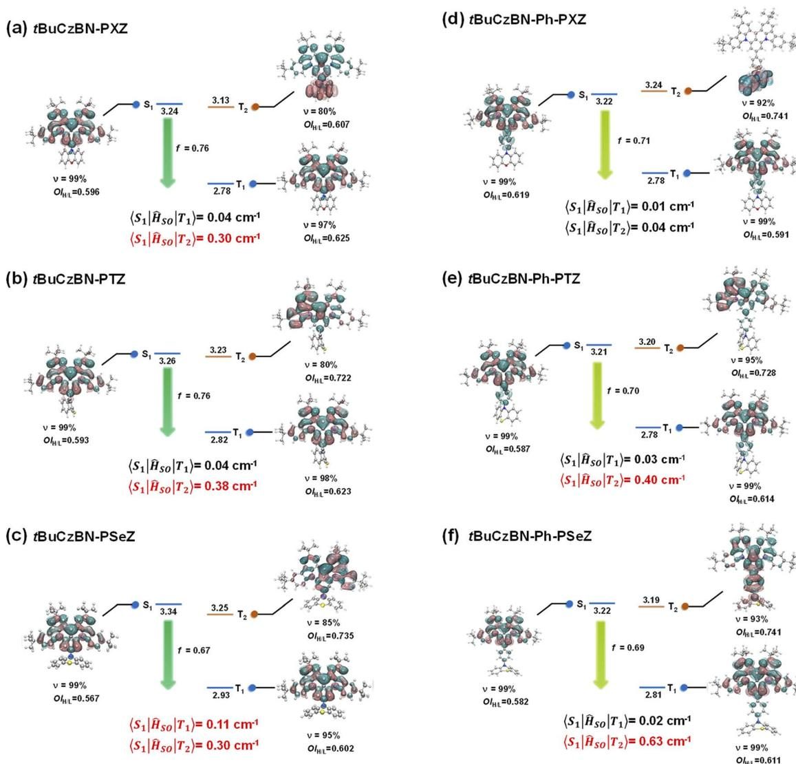
Fig. 5 Calculated energy-level diagrams, NTO distributions, and associated spin-orbit coupling (SOC) matrix elements for (a) **tBuCzBN-PXZ**, (b) **tBuCzBN-PTZ**, (c) **tBuCzBN-PSeZ**, (d) **tBuCzBN-Ph-PXZ**, (e) **tBuCzBN-Ph-PTZ** and (f) **tBuCzBN-Ph-PSeZ**.
