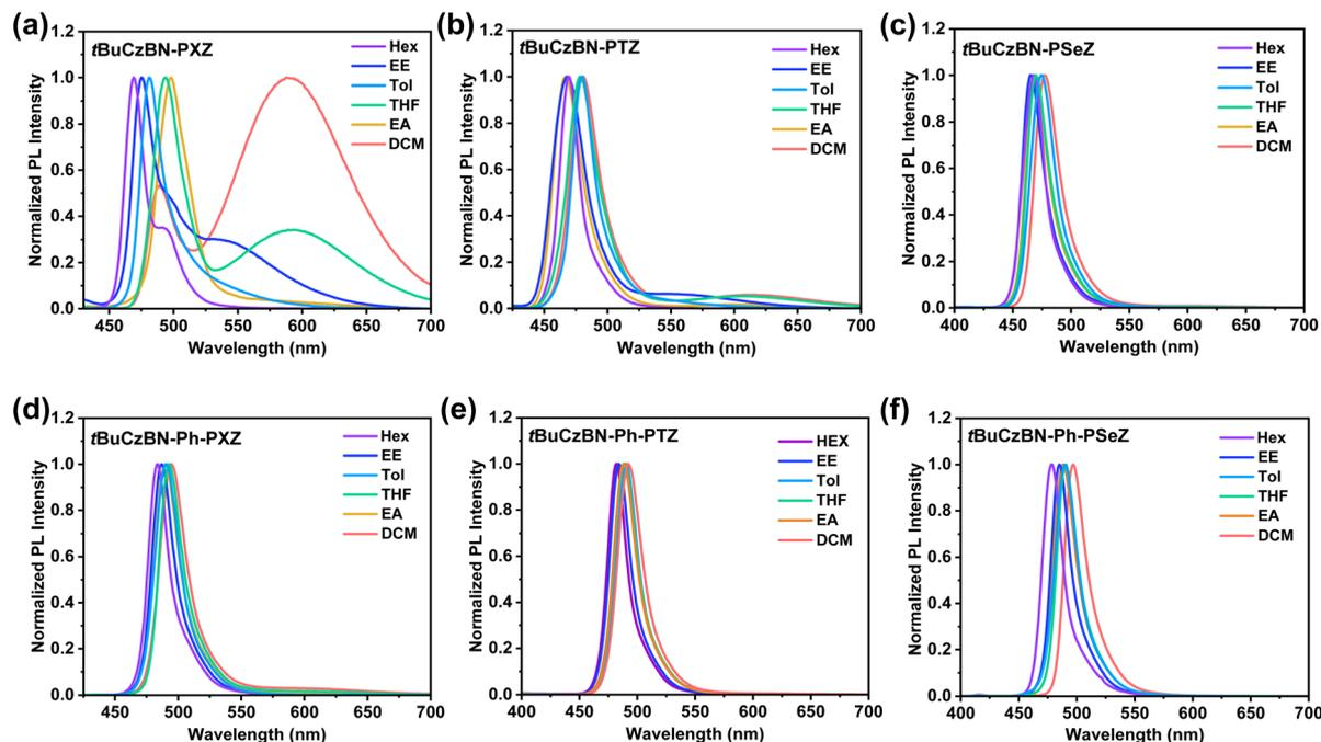
Fig. 3 Solvatochromic effect on PL spectra in  $10^{-5}$  M solution. (a) *t*BuCzBN-PXZ, (b) *t*BuCzBN-PTZ, (c) *t*BuCzBN-PSeZ, (d) *t*BuCzBN-Ph-PXZ, (e) *t*BuCzBN-Ph-PTZ and (f) *t*BuCzBN-Ph-PSeZ. Hex: *n*-hexane; EE: diethyl ether; Tol: toluene; THF: tetrahydrofuran; EA: ethyl acetate; DCM: dichloromethane.
