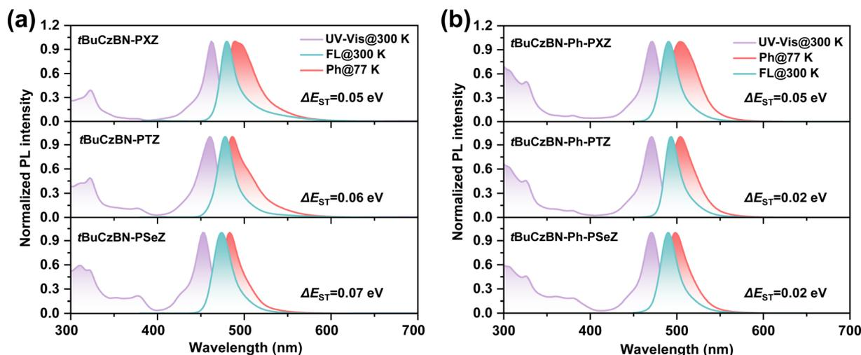
Fig. 2 The ultraviolet-visible absorption spectra and PL spectra of (a) **tBuCzBN-PXZ**, **tBuCzBN-PTZ**, and **tBuCzBN-PSeZ** diluted in toluene; (b) **tBuCzBN-Ph-PXZ**, **tBuCzBN-Ph-PTZ**, and **tBuCzBN-Ph-PSeZ** diluted in toluene.
