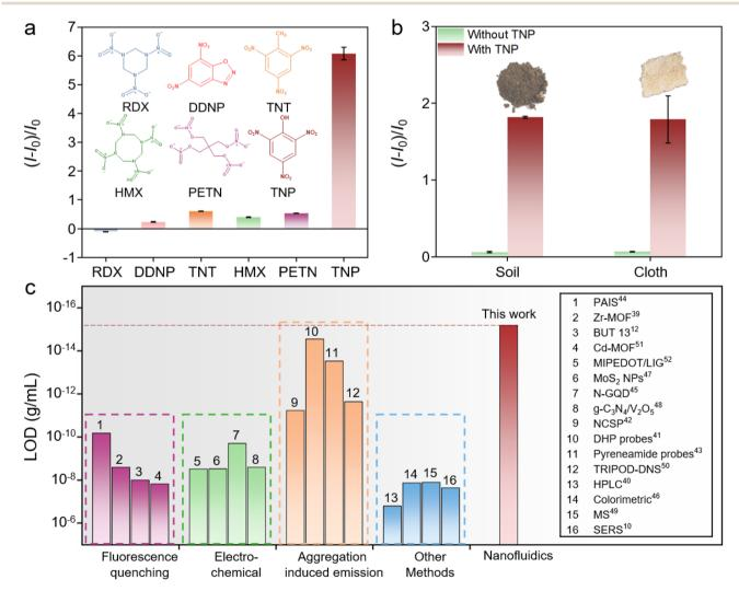
Fig. 4 Application viability of AAO@UiO-66-NH $_2$  for TNP detection. (a) Comparing the detection performance of different explosives (concentrations are all  $10^{-10}$  g mL $^{-1}$ ). (b) Testing of explosives in the actual environment (soil and cloth). (c) Comparison with the LOD of the reported sensors in the literature. $^{10.12,39-52}$
