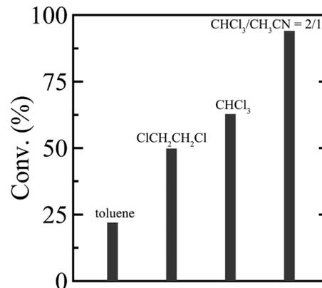
**Fig. 1** Solvent effect on the postpolymerization reaction of P(St<sub>0.8-co</sub>-StOH<sub>0.2</sub>) with 2FPy<sup>+</sup>-CH<sub>2</sub>-C<sup>-</sup>Tf<sub>2</sub>.
