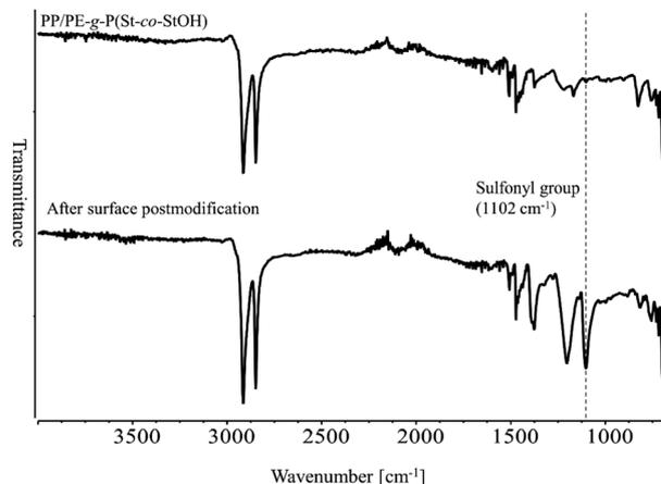
Fig. 6 Attenuated total reflectance-mode Fourier transform infrared spectra of membranes prior to (upper) and after (lower) the surface reaction of PE/PP-*g*-P(St-*co*-StOH) with  $2\text{FPy}^+\text{-CH}_2\text{-C}^-\text{Tf}_2$ .
