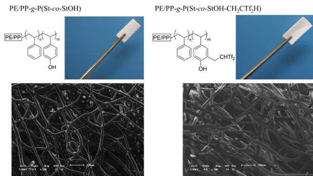
Fig. 7 Optical image (upper) and scanning electron microscopy (lower) images of membranes prior to and after the surface reaction of PE/PP-g-P(St-co-StOH) with  $2\text{FPy}^+-\text{CH}_2-\text{C}^-\text{Tf}_2$ .
