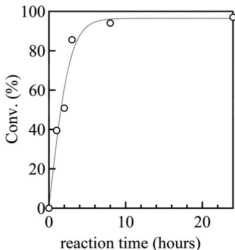
Fig. 2 Kinetic plots of the postpolymerization reaction of P(St<sub>0.8</sub>-co-StOH<sub>0.2</sub>) with 2FPy<sup>+</sup>-CH<sub>2</sub>-C<sup>-</sup>Tf<sub>2</sub> (the dashed line is an eye guide).
