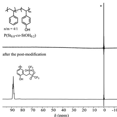
Fig. 4 The <sup>19</sup>F nuclear magnetic resonance spectra in CDCl<sub>3</sub> of the polymers prior to (upper) and after (lower) the postpolymerization reaction of P(St<sub>0.8</sub>-co-StOH<sub>0.2</sub>) with 2FPy<sup>+</sup>-CH<sub>2</sub>-C<sup>-</sup>Tf<sub>2</sub> (\* refers to the internal reference, C<sub>6</sub>F<sub>6</sub>).
