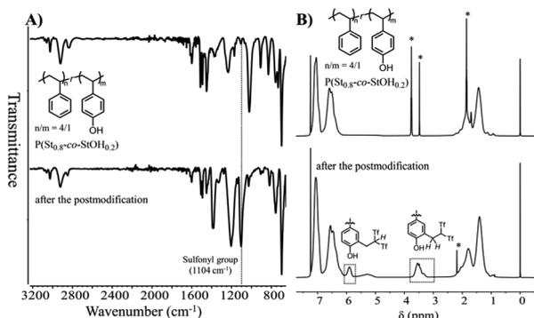
Fig. 3 Attenuated total reflectance-mode Fourier transform infrared spectra (A) and <sup>1</sup>H nuclear magnetic resonance spectra in CDCl<sub>3</sub> (B) of polymers prior to (upper) and after (lower) the postpolymerization reaction of P(St<sub>0.8</sub>-co-StOH<sub>0.2</sub>) with 2FPy<sup>+</sup>-CH<sub>2</sub>-C<sup>-</sup>Tf<sub>2</sub> (\* refers to the residual solvents).
