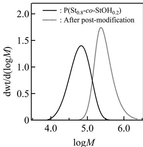
Fig. 5 Size-exclusion chromatography measurements of the polymers prior to (solid) and after (dashed) the postpolymerization reaction of  $P(\text{St}_{0.8}\text{-co-StOH}_{0.2})$  with  $2\text{FPy}^+\text{-CH}_2\text{-C}^-\text{Tf}_2$ . The measurement condition was  $0.35\text{ mL min}^{-1}$  in dimethylformamide (DMF) containing  $0.01\text{ mol L}^{-1}$  LiCl at  $40\text{ }^\circ\text{C}$ .
