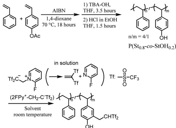
**Scheme 2** Schematic overview of the synthesis of polymers bearing Tf<sub>2</sub>CH<sub>2</sub> derivatives *via* postpolymerization reactions of polymeric phenol derivatives with 2FPy<sup>+</sup>-CH<sub>2</sub>-C<sup>-</sup>Tf<sub>2</sub>.
