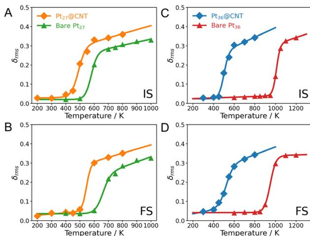
Fig. 5 Phase transition behaviors of  $\text{Pt}_{27}$  and  $\text{Pt}_{36}$  inside CNT as well as bare clusters at the IS (A and C) and FS (B and D). The calculated values are represented by points, and the corresponding fitted curves are shown by lines.
