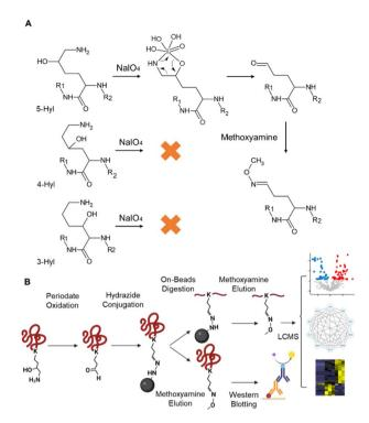
Fig. 1 Constitutional isomer selective enrichment and analysis of protein 5-Hyl modification. (A) Chemistry of the constitutional isomer selective reaction of protein lysine 5-hydroxylation. (B) Enrichment and analysis workflow to systematically profile protein 5-Hyl modification
