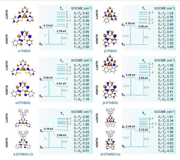
Fig. 3 Natural transition orbital distributions (HONTO and LUNTO) of  $S_1$  states, and spin-orbit coupling matrix element (SOCME) for the emitters calculated using the TD-DFT method at M062X/def2SVP level.
