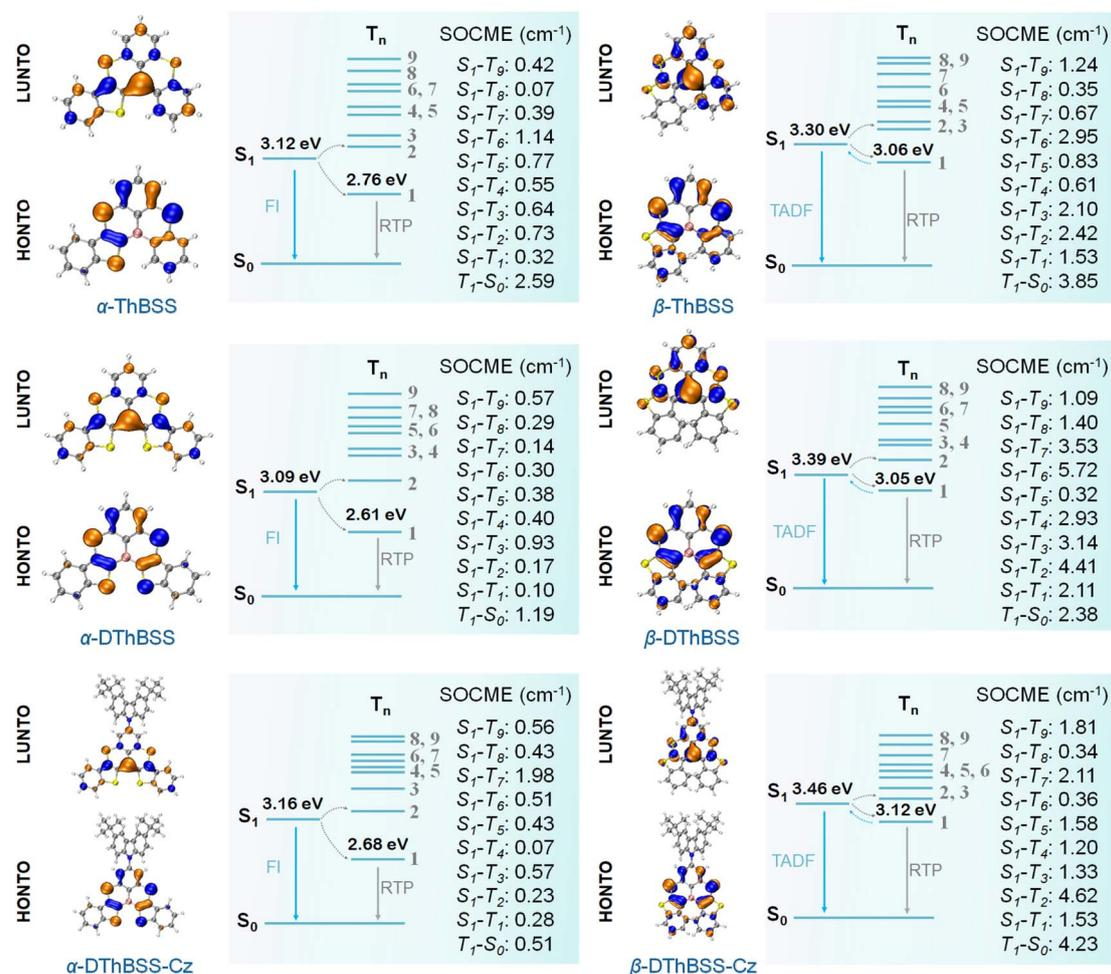
Fig. 3 Natural transition orbital distributions (HONTO and LUNTO) of  $S_1$  states, and spin-orbit coupling matrix element (SOCME) for the emitters calculated using the TD-DFT method at M062X/def2SVP level.
