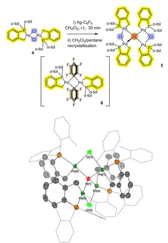
Fig. 3 Formation of Pd<sub>4</sub> cluster 5 from palladacycle 4. The single crystal XRD structure of 5 is shown with selected ellipsoids (set to 50%) for clarity (all H-atoms, with the exception of the bridging-hydroxo ligands, have been hidden from view). Selected interatomic lengths/Å: Pd1-Cl1 = 2.4737(8), Pd1-O1 = 2.101(2), Pd1-P1 = 2.2093(9), Pd1-Cl = 2.052(3). Selected interatomic angles/°: Pd1-Cl1-Pd2 = 84.35(3), Pd3-Cl2-Pd4 = 84.67(3), Pd1-O1-Pd4 = 103.46(9), Pd2-O1-Pd3 = 113.65(10)
