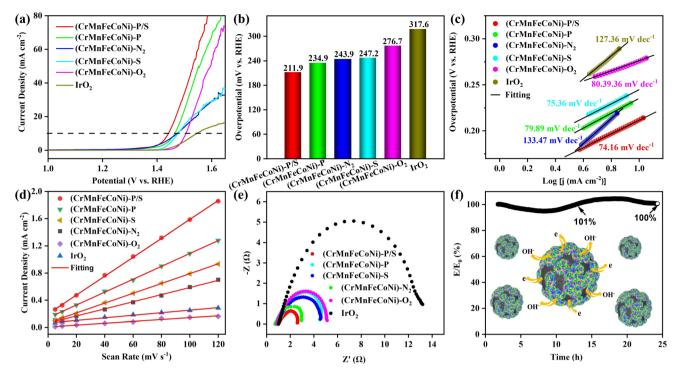
Fig. 4 OER performance: (a) LSV curves; (b) overpotentials at  $10 \text{ mA cm}^{-2}$ ; (c) Tafel slopes; (d) the current density against scan rates for estimating C<sub>dl</sub> values and (e) EIS spectra of the (CrMnFeCoNi)-P/S, (CrMnFeCoNi)-P, (CrMnFeCoNi)-N<sub>2</sub>, (CrMnFeCoNi)-S, (CrMnFeCoNi)-O<sub>2</sub> and  $IrO_2$  electrodes. (f) Long-time stability test of the HEM-HENMC at 20 mA cm<sup>-2</sup> for 25 h.
