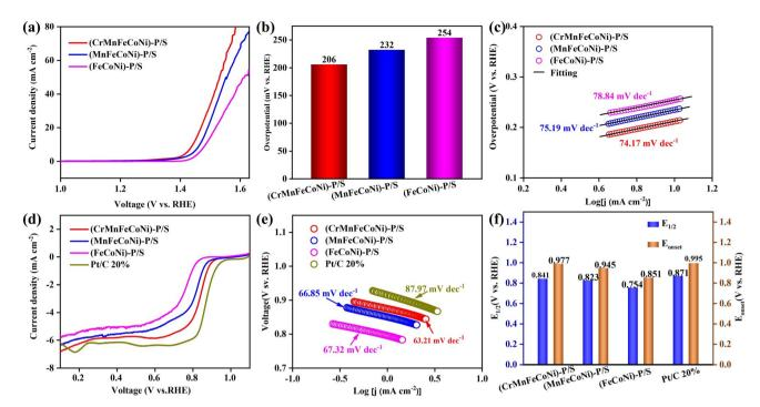
Fig. 5 OER performance. (a) LSV curves; (b) overpotentials at 10 mA cm $^{-2}$  and (c) Tafel slopes of the (CrMnFeCoNi)-P/S, (MnFeCoNi)-P/S, and (FeCoNi)-P/S electrodes. ORR performance. (d) LSV curves, (e)  $E_{1/2}$  and  $E_{onset}$  (vs. RHE) and (f) Tafel slopes of the (CrMnFeCoNi)-P/S, (MnFeCoNi)-P/S, (FeCoNi)-P/S and Pt/C 20% electrodes.
