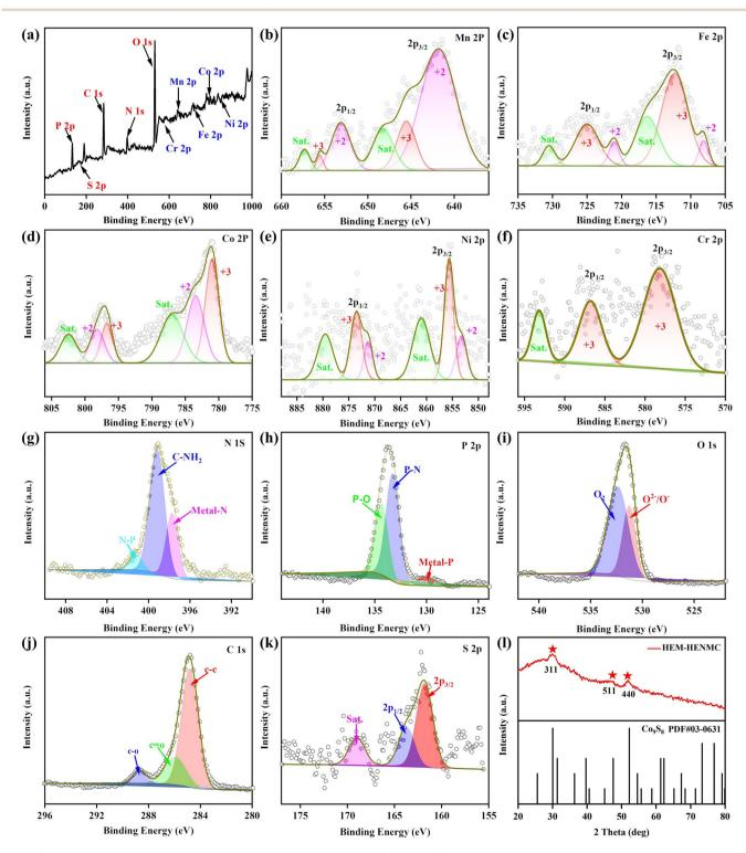
Fig. 3 (a) Full XPS survey spectrum; (b–k) high-resolution XPS spectra of (b) Mn 2p, (c) Fe 2p, (d) Co 2p, (e) Ni 2p, (f) Cr 2p, (g) N 1s, (h) P 2p, (i) O 1s, (j) C1s and (k) S 2p for the HEM–HENMC; and (l) XRD pattern of the HEM–HENMC.
