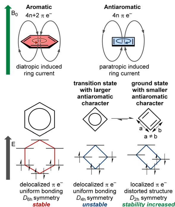
Fig. 1 Key features differentiating aromatic and antiaromatic compounds exemplified by a benzene ring and a cyclobutadiene ring.  $B_0$  denotes the direction of an external magnetic field inducing ring current in the (anti)aromatic compounds.
