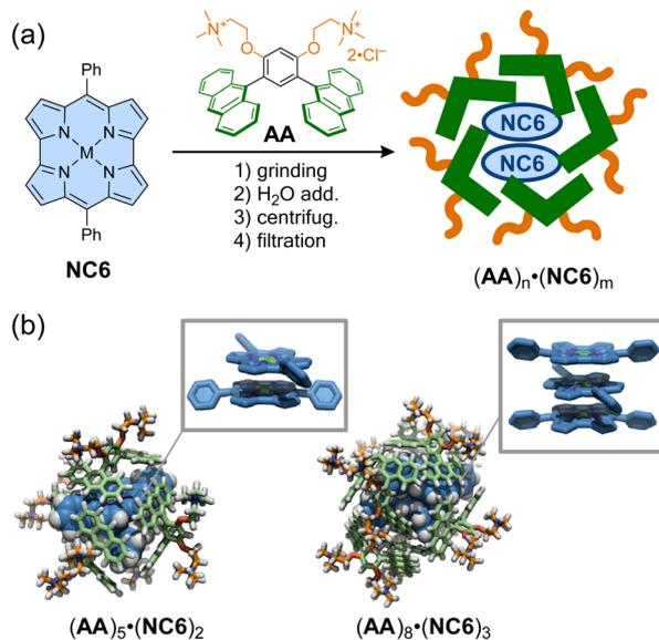
Fig. 9 (a) Encapsulation of *meso*-phenyl Ni(II)-norcorrole (NC6) within anthracene-based micellar capsules to form  $(AA)_n \cdot (NC6)_m$ . (b) Optimized structures of  $(AA)_5 \cdot (NC6)_2$  and  $(AA)_8 \cdot (NC6)_3$  and their highlighted guest stacking. The color scheme for the models: H (white), C (blue, pale green, and orange), N (dark blue), and Ni (green).
