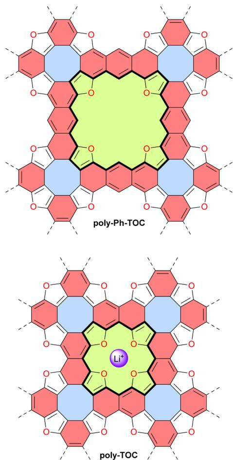
Fig. 13 Tetraoxa[8]circulene-based 2D polymers **poly-Ph-TOC** and **poly-TOC**. The binding site of **poly-TOC** for  $\text{Li}^+$  is indicated. Different subunits are colored as follows: blue for antiaromatic cyclooctatetraene, red for aromatic anthracene or naphthalene, and green for potentially antiaromatic extended and normal tetraoxaisophlorin with 28 and 20  $\pi$ -electron circuits indicated in bold.
