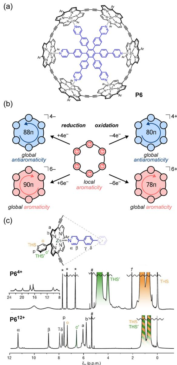
Fig. 10 (a) Chemical structure of the porphyrin nanoring P6. (b) Expression of global aromaticity/antiaromaticity of P6 induced by redox reactions; the arrows indicate the direction of the ring current induced by a magnetic field perpendicular to the plane directed toward the observer. (c) <sup>1</sup>H NMR spectra (500 MHz,  $CD_2Cl_2$ , 223 K) of P6<sup>4+</sup> (top) and P6<sup>12+</sup> (bottom).
