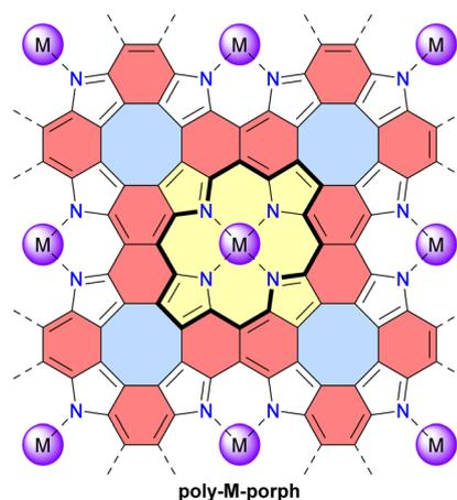
Fig. 14 Structure of the metalloporphene (single-layered) and metalloporphite (multi-layered) 2D polymers **poly-M-porph**. Different subunits are colored as follows: blue for antiaromatic cyclooctatetraene, red for aromatic naphthalene, and yellow for aromatic porphyrin with the 18  $\pi$ -electron circuit indicated in bold.
