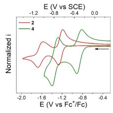
Fig. 2 Normalized cyclic voltammograms of 2 (red line) and 4 (green line). Experimental conditions: 1 mM of 2 or 4, 0.1 M TBAPF $_6$  supporting electrolyte in degassed THF. WE: glassy carbon. Pseudo RE: Ag wire (ferrocene as internal reference). CE: Pt wire. Scan rate, 100 mV  $_6^{-1}$
