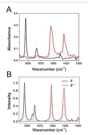
Fig. 4 Experimental (A) and calculated (B) IRSEC spectra of 2 recorded under reductive polarization. Black traces represent the spectra of the neutral species (no polarization), red spectra show the resulting reduced species after bulk electrolysis, and grey traces display intermediate situations. Solvent: dry THF, 0.1 M TBAPF<sub>6</sub>. The computed frequencies were scaled by 0.983.
