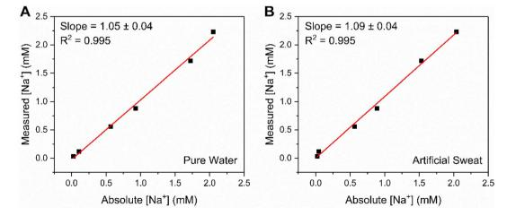
Fig. 6 Correlation plot showing the excellent agreement between absolute and measured [Na<sup>+</sup>] values at B15C5<sub>SAM</sub>, for a range of unknown concentrations (up to 3 mM) in (A) pure water (100 mM TEACl) and (B) a simple, artificial sweat matrix (100 mM TEACl, 11.3 mM lactic acid, 21.6 mM urea in pure water). Measured [Na<sup>+</sup>] values were estimated from fitting a Langmuir–Freundlich model (eqn (S2)†) to a prior obtained calibration curve.
