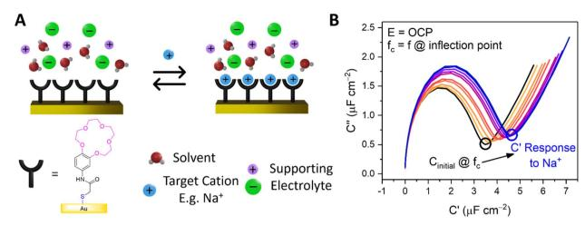
Fig. 1 (A) Schematic depiction of  $B15C5_{SAM}$  in the absence (left) and presence (right) of a specific target. (B) Capacitive Nyquist plots of  $B15C5_{SAM}$  in H<sub>2</sub>O, 100 mM TEACI conducted at fixed OCP. Changes in C are measured at the inflection point of each Nyquist plot (corresponding to frequency,  $f_c$ ) upon addition of increasing concentrations of NaCl up to 50 mM (blue) in static solution.
