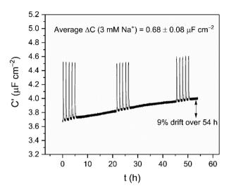
Fig. 5 Long term cation sensing experiment conducted over 54 h in water (100 mM TEACl as supporting electrolyte). Responses of  $B15C5_{SAM}$  to 3 mM Na<sup>+</sup> are shown as spikes in the sensogram.
