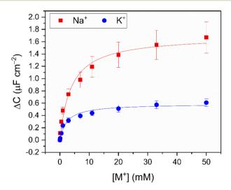
**Fig. 2** Response isotherms of **B15C5<sub>SAM</sub>** determined from the shift in C' in response to increasing concentrations of Na<sup>+</sup> (red squares) and K<sup>+</sup> (blue circles) in H<sub>2</sub>O with 100 mM TEACl as supporting electrolyte, under static conditions. Isotherms were fitted to a Langmuir model (see ESI Section S1.6 for further details, and eqn (S1)†). Errors represent one standard deviation of three independent repeats.
