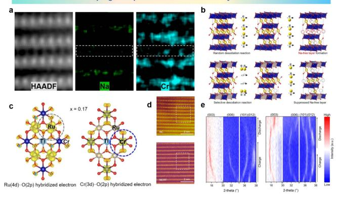
Ru/Ti co-doping manipulated electron orbital hybridization mode
