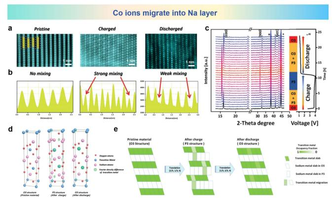
Fig. 6 (a) The STEM images and (b) corresponding line profiles of the NCT electrode at pristine (left), fully charged (middle) and fully discharged (right) stages. (c) *In operando* XRD patterns measured at 10 mA  $g^{-1}$  and phase evolution during cycling. (d) Density difference electron density maps for different states produced by Fourier transforms. (e) Schematic plot of reversible TM migration upon cycling. (a)–(e) are reprinted with permission from ref. 105. Copyright 2019 Wiley.
