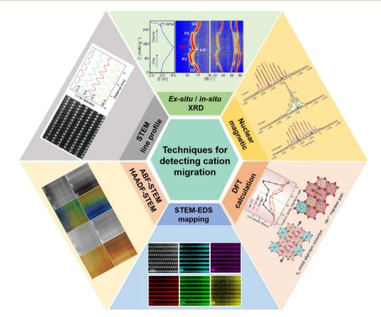
Fig. 22 Advanced characterization techniques for detecting cation migration.
