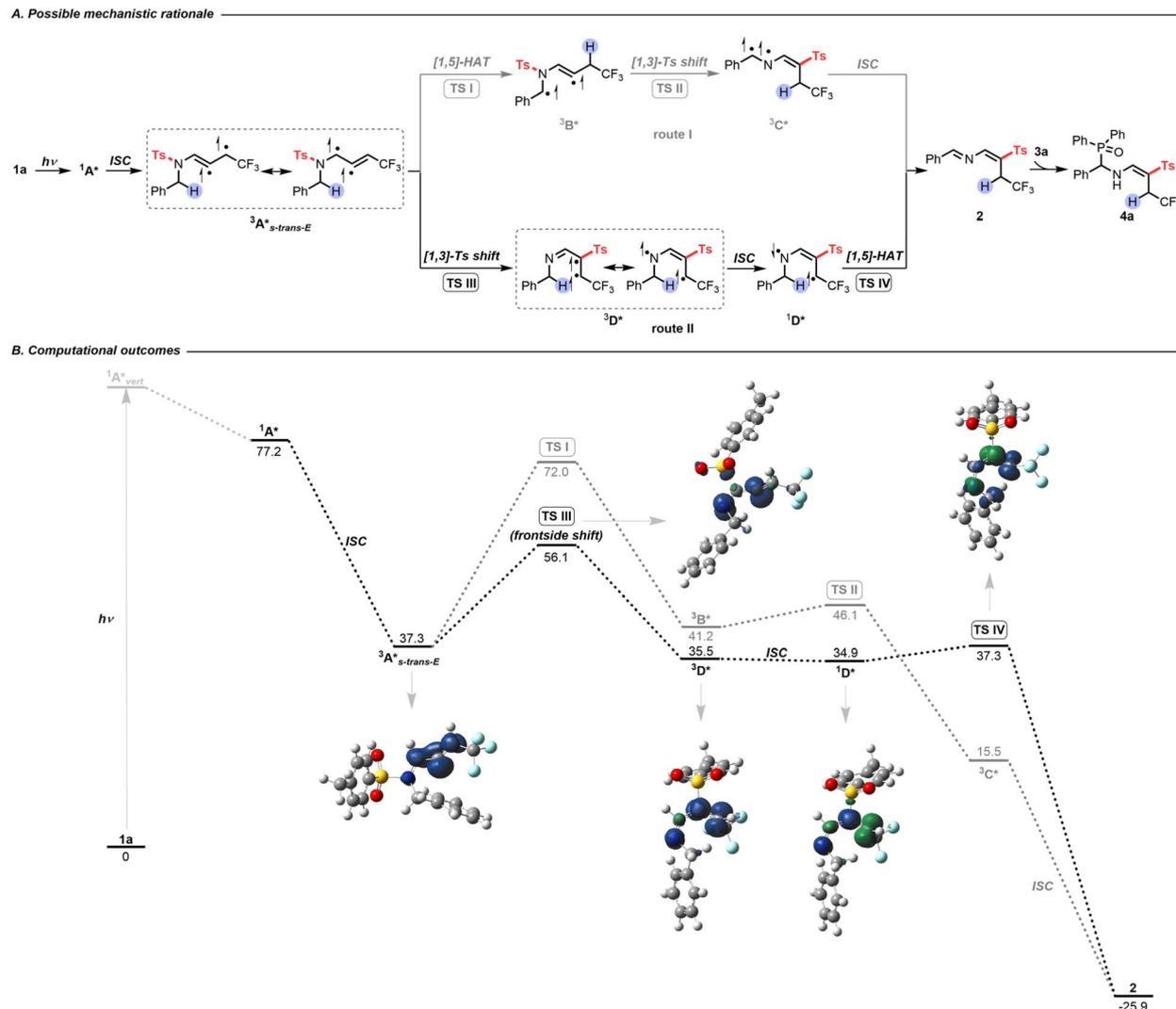
**Scheme 3** (A) Possible mechanistic rationale. (B) Computational outcomes. Gibbs free energies ( $\text{kcal mol}^{-1}$ ) were computed at the PBE0/6-311++G(d,p) level of theory using DMSO as an implicit solvent with the PCM method. Spin densities are reported for the triplet and singlet diradical states (isocontour value 0.01 au).
