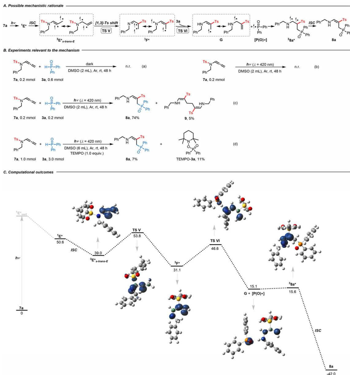
**Scheme 4** (A) Possible mechanistic rationale. (B) Experiments relevant to the mechanism. (C) Computational outcomes. Gibbs free energies ( $\text{kcal mol}^{-1}$ ) computed at the PBE0/6-311++G(d,p) level of theory using DMSO as an implicit solvent with the PCM method. Spin densities are reported for the triplet and singlet diradical states (isocontour value 0.01 au).
