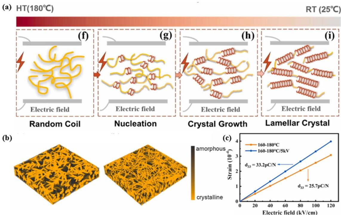
Fig. 10 (a) Schematic diagram showing the proposed mechanism for *in situ* electrostatic field regulating the recrystallization behaviors of P(VDF-TrFE) films. (b) Simulation microstructure models of (left) 160–180 °C and (right) 160–180 °C/5 kV P(VDF-TrFE) films. (c) The simulated average strain–electric field line plot for the two microstructures. This figure has been reproduced from ref. 125 with permission from Elsevier, copyright 2022.
