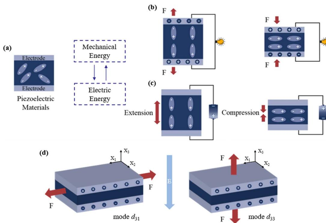
Fig. 2 Schematic diagram showing (a) the mechanism of piezoelectric materials; (b) direct piezoelectric effect; (c) converse piezoelectric effect. This figure has been reproduced from ref. 36 with permission from American Chemical Society, copyright 2023. (d) Operating modes of a piezoelectric material: mode  $d_{31}$  (left) and mode  $d_{33}$  (right).
