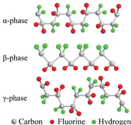
Fig. 3 Schematic diagram showing the chain conformations of  $\alpha$ ,  $\beta$  and  $\gamma$  phases in PVDF. This figure has been reproduced from ref. 66 with permission from John Wiley and Sons, copyright 2018.
