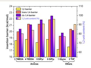
Fig. 5 Comparison of minimal energy barriers (calculated at wB97X-2-D3(BJ)/def2-QZVPP level) for 1,2, cis-1,4 and trans-1,4 butadiene additions with various Lewis bases, including corresponding 1,2-unit content data from polymerization experiments.
