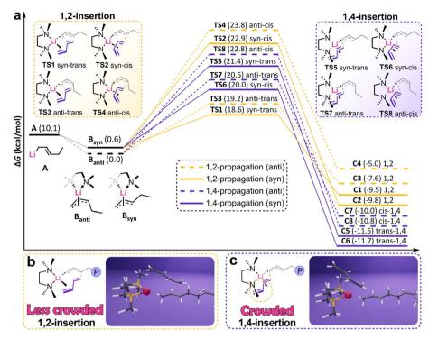
Fig. 4 (a) Energy profile of butadiene anionic polymerization with TMEDA as ligand and potential transition states. (Energies were calculated at ωB97X -2-D3(BJ)53/def2-QZVPP level) (b) and (c) Visualizing how steric hindrance influences energy barriers of 1,2 and 1,4-additions.
