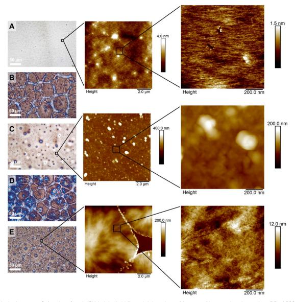
Fig. 4 Optical microscopy (left column) and AFM height (middle and right columns) images of homopolyamines with a DP of 300 and block copolymers with a DP of 100. (A) Depicts a racemic polyamine  $\cdot$  HCl (P4), (B) depicts a R-configured polyamine  $\cdot$  HCl (P12), (D) depicts a block copolymer (R-50/S-50, P14) and (E) depicts a block copolymer (R-50/R-50, P17). Black squares represent zoom-in images.
