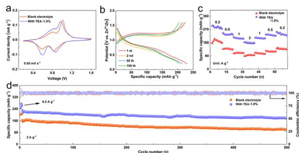
Fig. 5 (a) CV curves, (b) the voltage profiles, (c) rate capability and (d) long-term cycling performance of the Zn||V<sub>2</sub>O<sub>5</sub> batteries in the electrolytes with/without 1.0%-TEA additive.
